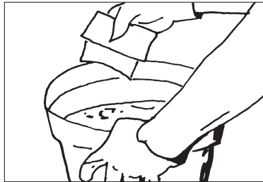
Water activate Leak Stop
