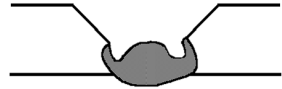
Groove welds are prone to undercut along the edges, increasing the risk of trapping slag when the next pass is made
