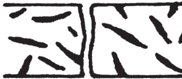
A crack in cast iron. The carbon flakes in the metal are saturated with oil.
