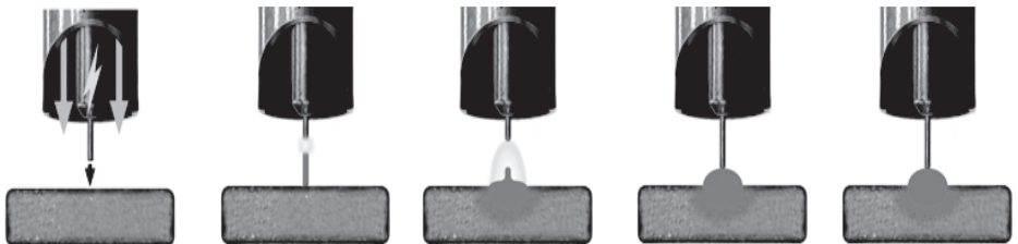
Short circuiting (short arc welding)
