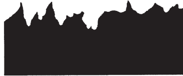
Structural peaks acting as attack points for corrosion
