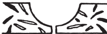
After gouging with Unitor CH-2. The oily deposits in the welding area have evaporated.
