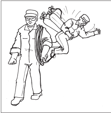
Keep cables and hoses clear of passage ways.
