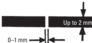
Close square butt joint
