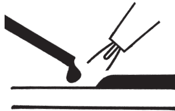
Gas weld Leftward. Note that the weld pool must not be stirred with the filler rod
