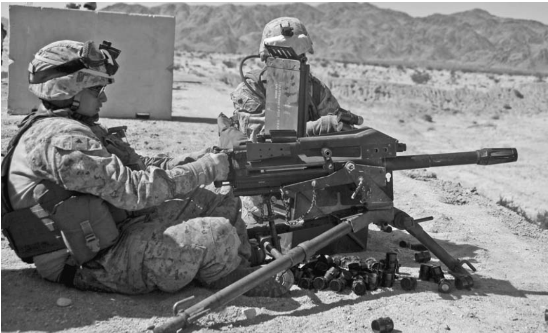
The U.S. Mk 19 Mod 3 40 × 53mm automatic grenade launcher. This weapon is capable of providing devastating fire support to almost 2000 yards (Pfc. J.A. Ortiz, U.S. Marine Corps).
