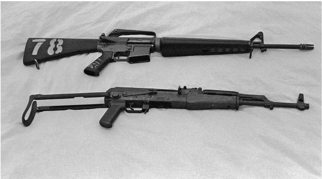
5.56mm M16A1 (top) compared to the 7.62mm AKMS. The flash hider on the M16 is the early pattern open prong type. Later models were closed to prevent snagging on foliage (Sgt. B. Bethune, Department of Defense).
