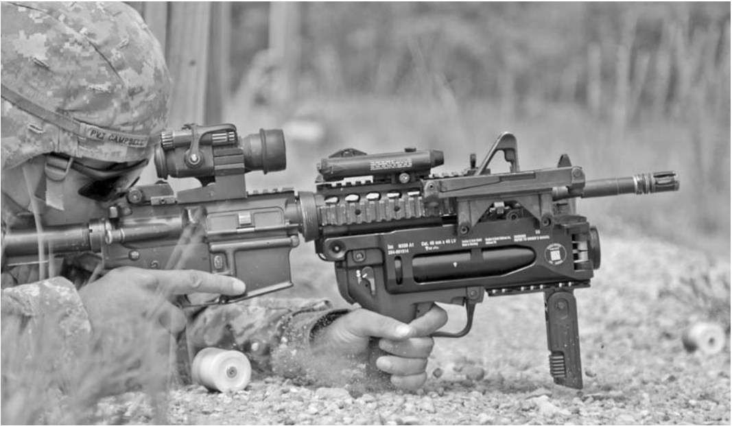
Above: The U.S. M320 40mm grenade launcher, the M203's replacement. This HK is similar to the same launcher as used on the German G36 rifle (Spc. M.J. MacLeod, U.S. Army). Below: A U.S. M32 6-shot 40mm grenade launcher. This gives troops a big boost in mobile firepower (Cpl. S. D. Corum, U.S. Marine Corps).
