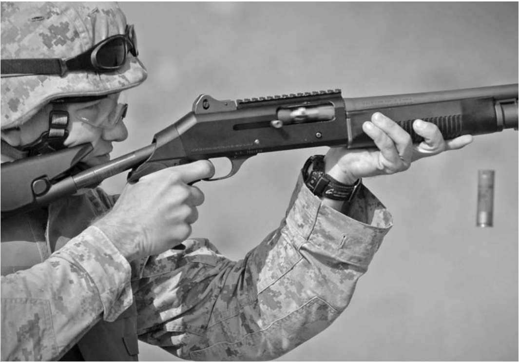
The U.S. M1014 semi-auto shotgun. This is the military designation for the Benelli M4 gas-operated design (MCC E.A. Clement, U.S. Navy).
