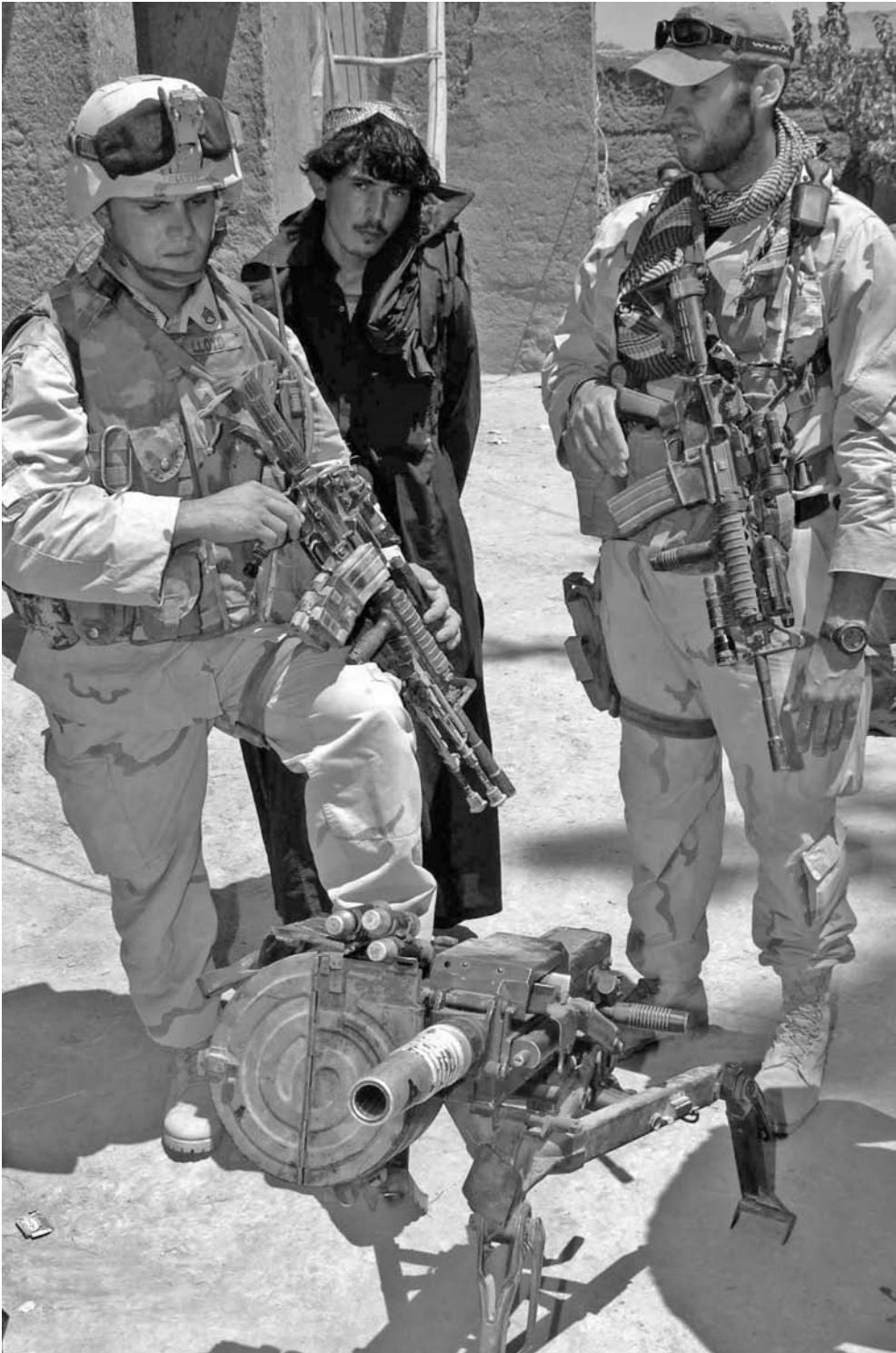
Russian AGS-17 30mm automatic grenade launcher; this was the Soviet answer to the Mk 19. There is an updated AGS-30 model still in service, though a new 40mm Russian design has recently been developed (Sgt. A. Reynolds, U.S. Army).
