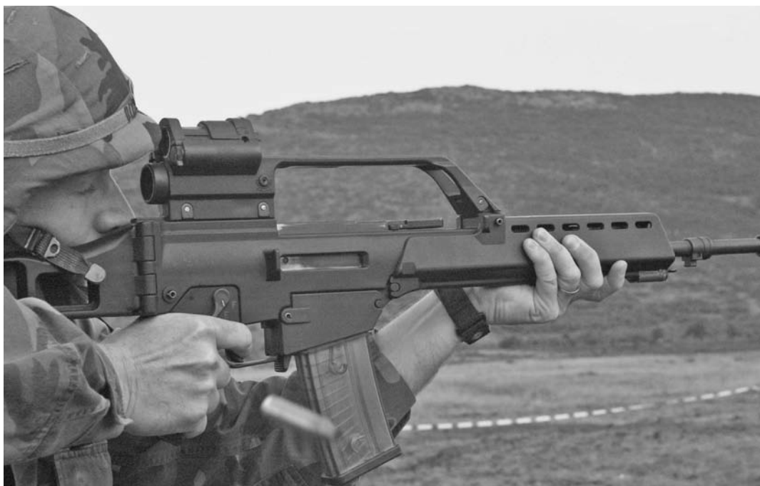
The new 5.56mm HK G36, which uses a gas operated action, unusual for HK designs (SFC J. Cervantez, U.S. Army).
