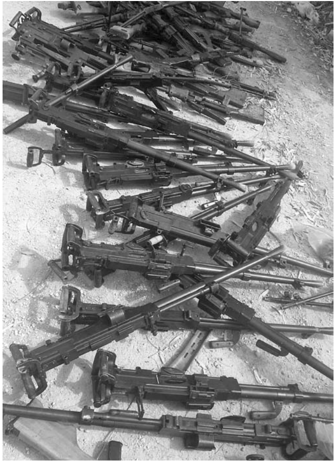
A mess of captured Russian made Iraqi 12.7mm NSV heavy machine guns. This model was a 1960s design meant to replace the DShKM, which it never fully did (GSgt. E.S. Hansen, U.S. Marine Corps).
