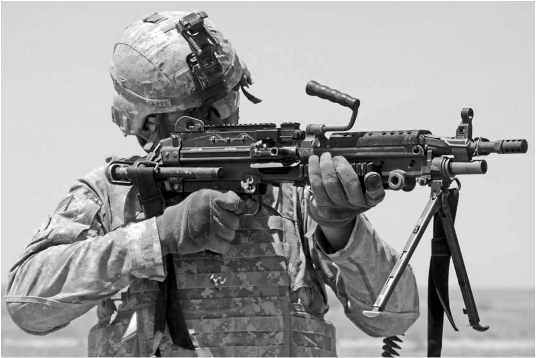
This is the 5.56mm U.S. M249 Para Squad Automatic Weapon. This variant uses a telescoping stock and short barrel to improve handling in tight quarters (Spc. E. Cabral, U.S. Army).
