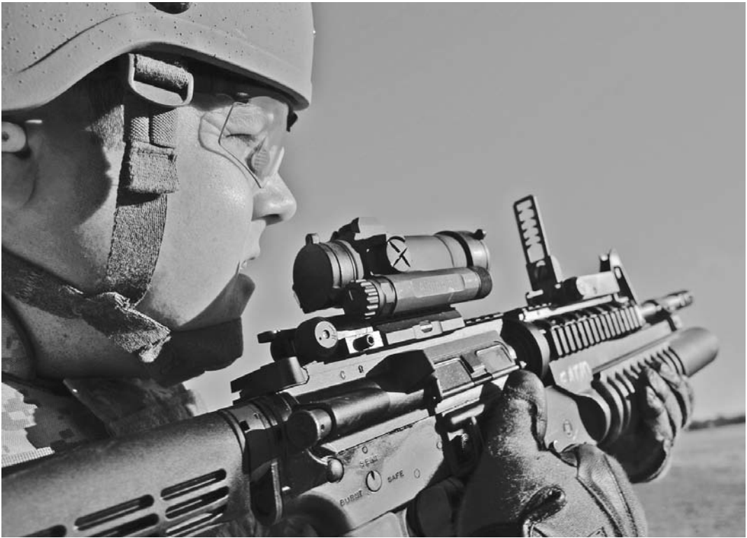
U.S. M203 40mm grenade launcher mounted below the M4 carbine (S. Thurow, U.S. Air Force).
