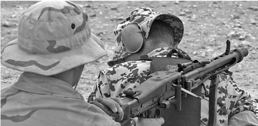
U.S. marine checking out a machine gun that first saw service under the Nazis, the German MG42. This is the modern 7.62mm NATO MG3 variation, which is still in production in several nations (SSgt. P. Bunting, U.S. Air Force).
