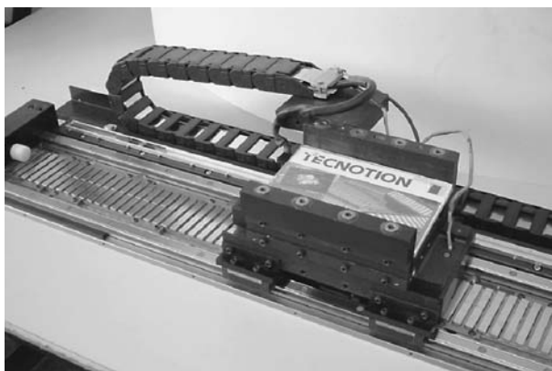
FIGURE 1.24 Linear motor. The magnets that cause the cogging are clearly visible.
