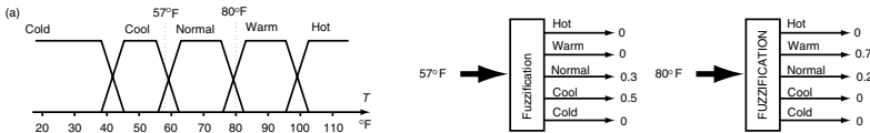
FIGURE 12.20 Fuzzification process: (a) typical membership functions for the fuzzification and the defuzzification processes, (b) example of converting a temperature into fuzzy variables.
