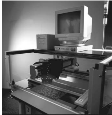
FIGURE 2.1 An optical inspection system for printed circuit boards. (Used by permission © CyberOptics Corporation 2001, all rights reserved.)
