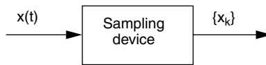
FIGURE 3.16 A continuous-time signal x(t) and a sampling device that produces a sample sequence \{x_k\} .
