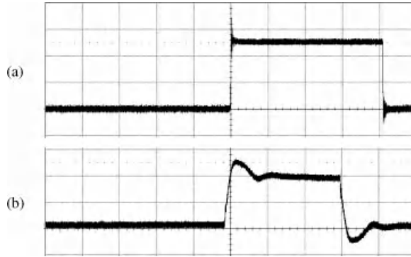
Figure 9.46 Waveforms: (a) inverter output voltage; (b) motor current for the drive with motor choke (scale 10\ \mu\text{s}/\text{div} , 200\ \text{V}/\text{div} – waveforms are not synchronized)
