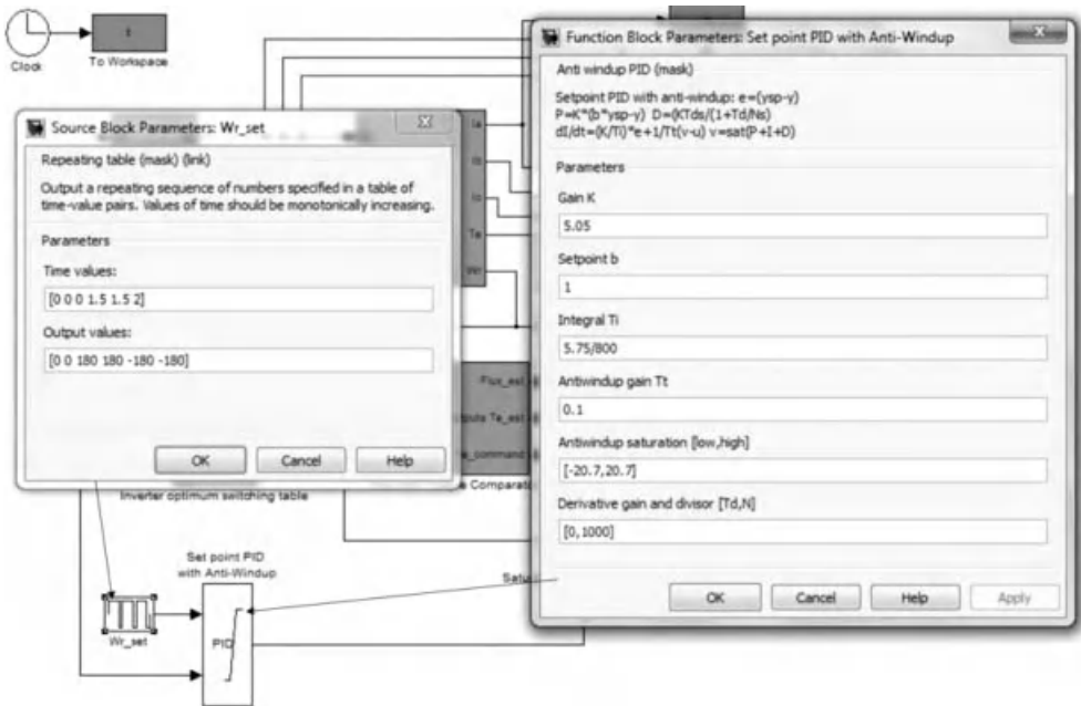
Figure 5.107 Speed command and parameters of PID controller
