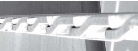
Figure 5.7 A Roebel bar. (a) Simplified presentation of two adjacent subconductors. (b), (c) Photographs illustrating the construction of a Roebel bar. A Roebel bar has minimal skin effect in a slot because of its perfect conductor transposition
