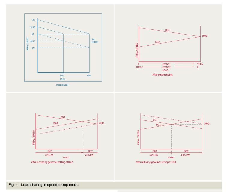
the power management system (PMS) compensates for the speed droop effect. Engine control governors do not have to be uniform in this control mode.
