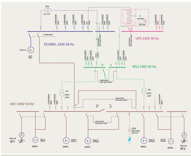
Fig. 2 – Low-voltage 690V network for auxiliary power station: diesel-mechanical propulsion.
