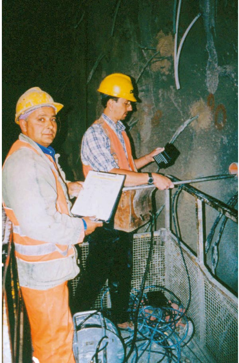
Taking core-face extrusion measurements using a sliding micrometer
