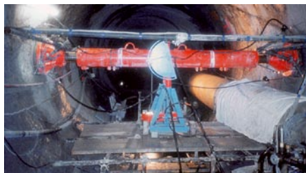
Loading and unloading test using a cylindrical jack
