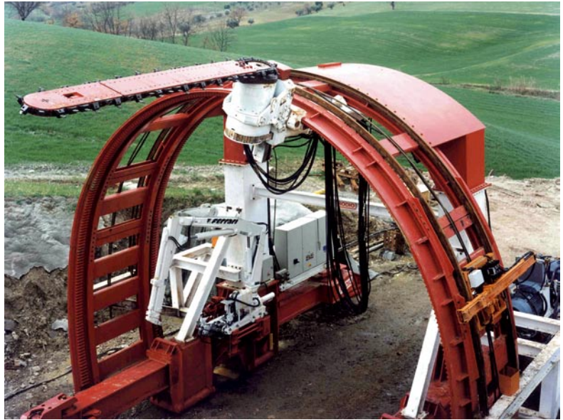
Cavity preconfinement by means of full face mechanical precutting: precutting machine constructed for the excavation of tunnels on the Sibari-Cosenza railway line (1985)
