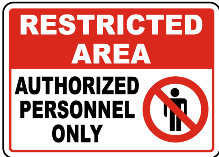
Figure 15 Example sign where battery systems are accessible. Required on the battery enclosure; or, all doors to the room/ fenced off section of a larger room where the battery system is accommodated
