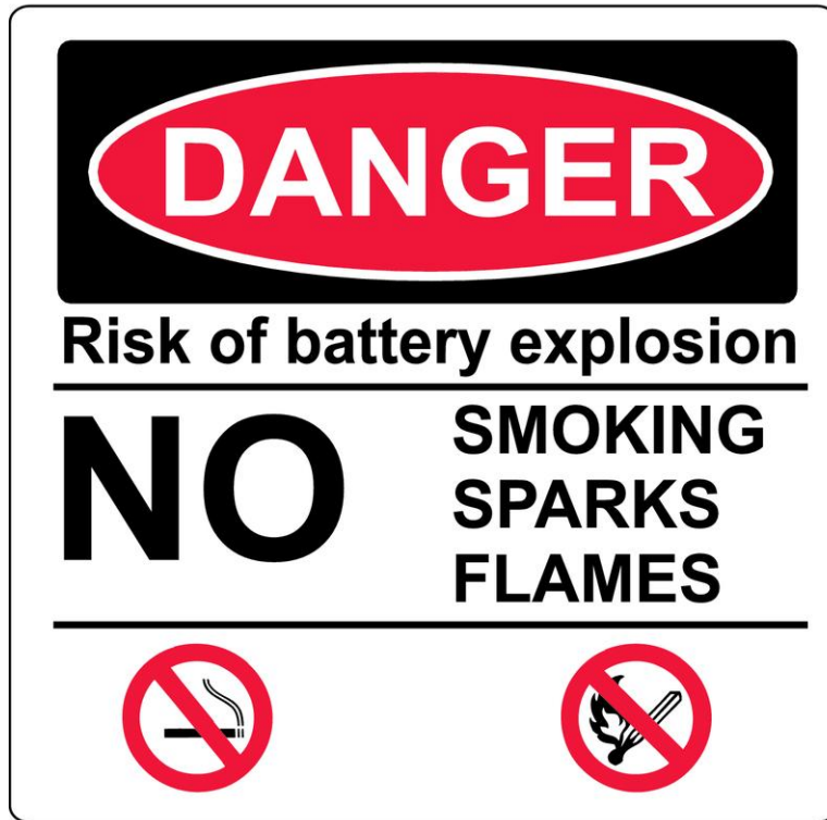
Figure 18 Example sign where explosive gas hazards apply. Required on enclosures, doors to battery rooms/ fenced off section of a larger room.
