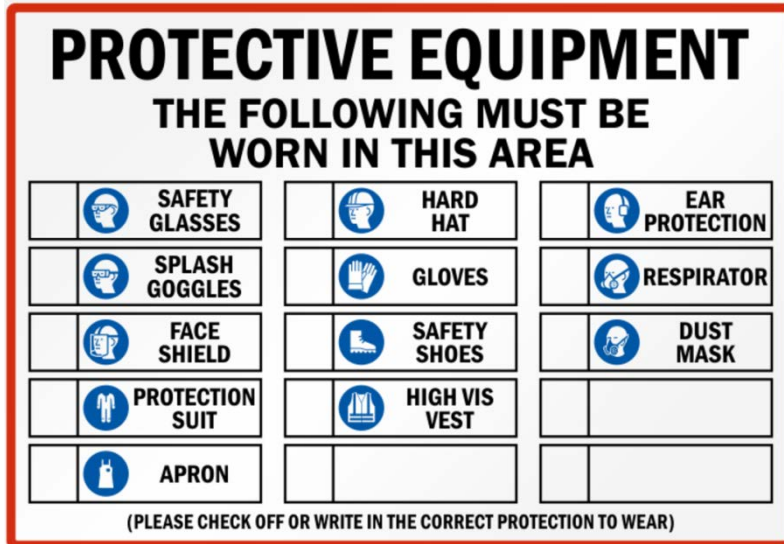
Figure 25 Example sign for battery systems where access requires personal protective equipment. The sign should be adjacent to the enclosure or on all doors to the room/ section of a larger room.
