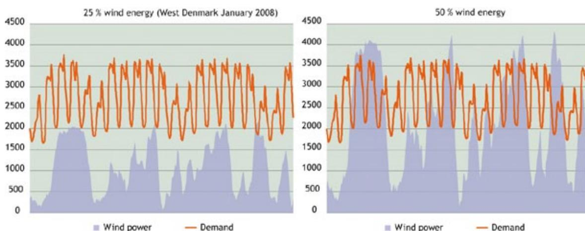
These charts show Demand (orange) and Wind Contribution (Blue shaded) overlaid. In the 25% penetration example, wind power peaks provide 100% of demand in West Denmark and no wind power is discarded. When reaching higher penetration levels, such as 50% (right side of chart), on infrequent occasions wind output must be curtailed in order not to exceed the demand.
