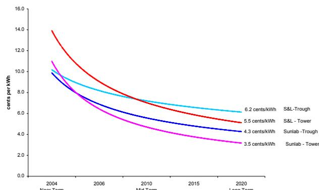
The red curve on the chart above represents the Sargent & Lundy cost projection for towers, while the mauve curve represents the SunLab tower projection. The main difference between the two projections is the cumulative installed capacity assumed by each. In the original report, these were referenced to an installation timeline from 2004–2020, but the more important factor in achieving the cost reductions was not the timeline but the total installed capacity.
