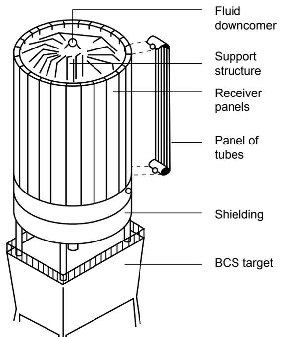
A receiver showing the tubes through which the molten salt passes<sup>16</sup>.
