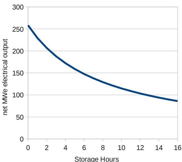
A graphical comparison of plant capacity (turbine size) and storage for the same mirror field size.
