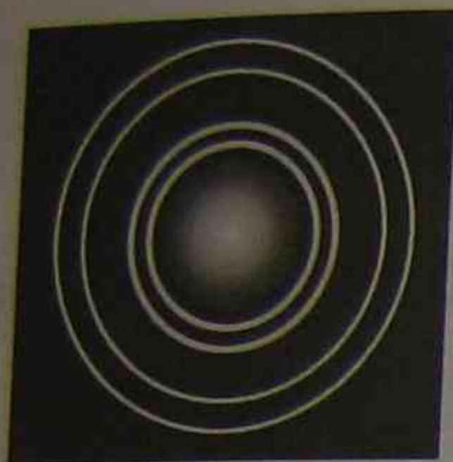
Figure 6.18 Electron diffraction pattern formed when a beam of electrons is passed through a thin metal foil
