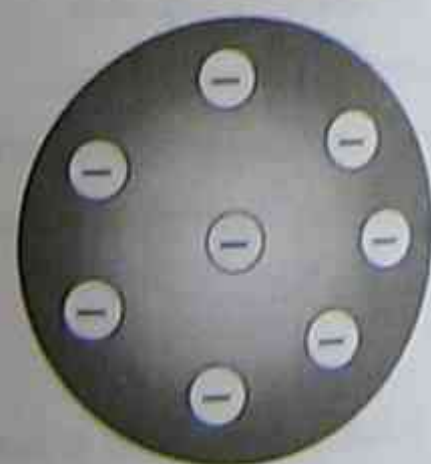
Sphere of positive electricity with electrons embedded like 'plums in a pudding'
