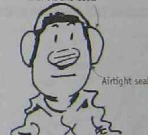
Figure 3.9 The structure of earmuffs showing how the sound waves are stopped from reaching the inner ear
