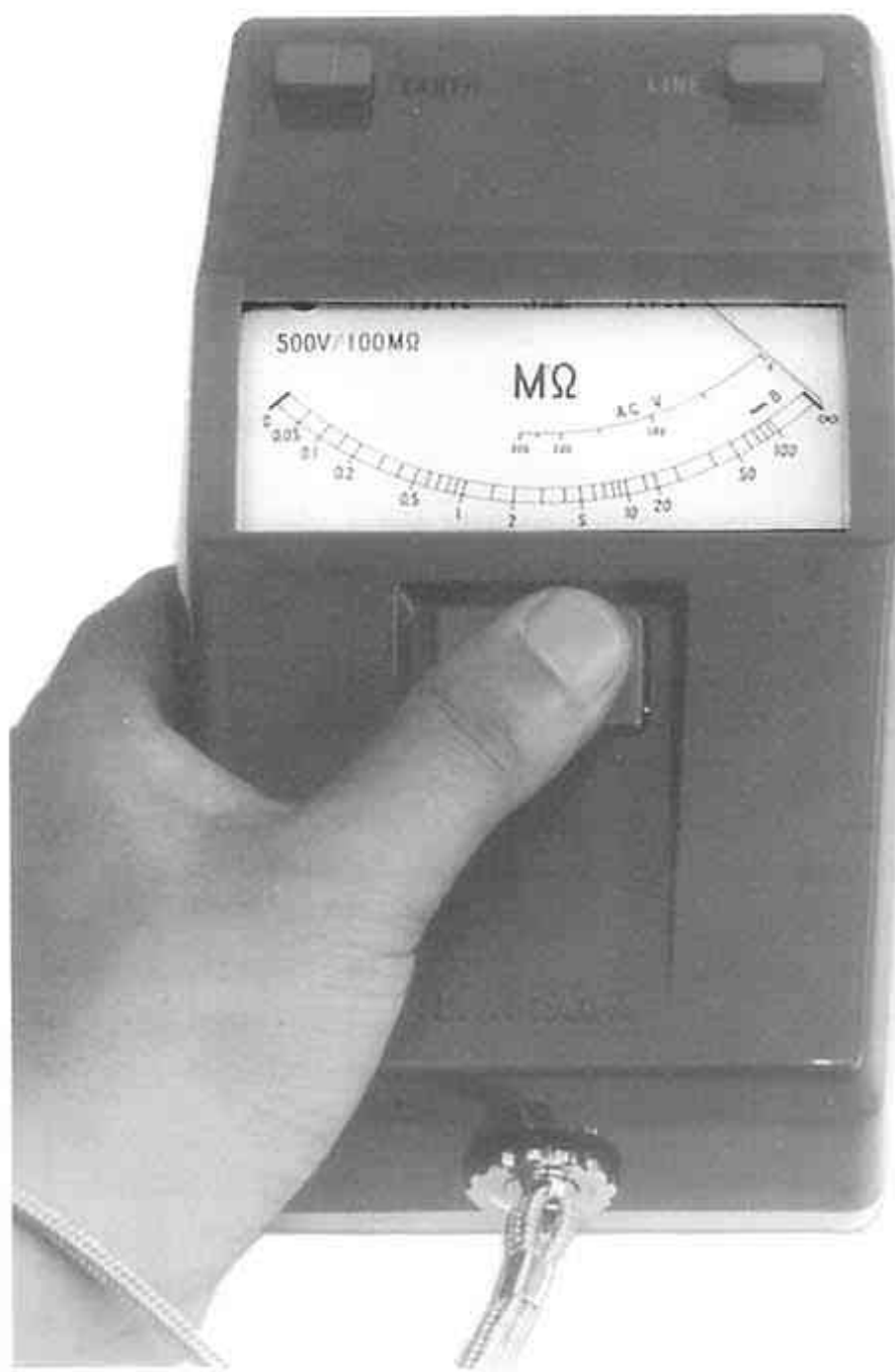
Fig. 11.15 This battery-operated insulation-resistance tester is light and compact
