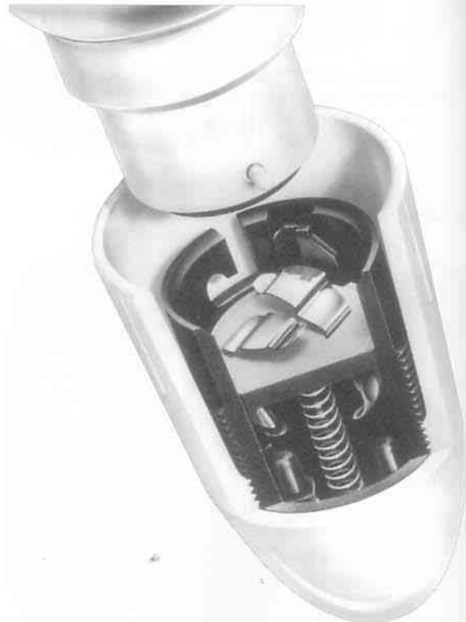
Fig. 5.38(e) Safety BC lampholder. Also available as a batten holder. Terminals become live only after a light bulb or BC adaptor is fitted HPM INDUSTRIES
