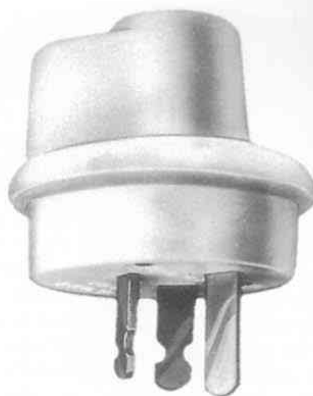
Fig. 5.37(d) Three-pin suppressor plug designed to reduce mains-borne electromagnetic interference caused by the switching of thermostatically controlled appliances GERARD INDUSTRIES
