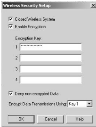
Figure B.7 Lucent's AP-1000 proprietary security mechanism.
