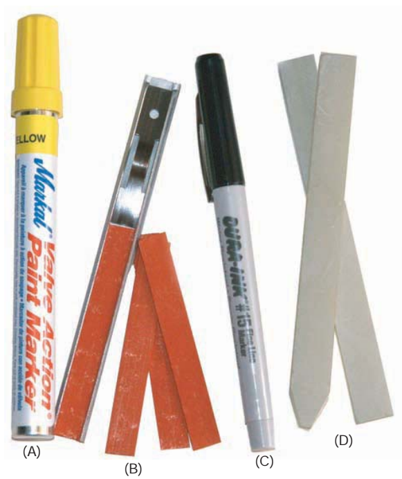
FIGURE 6-15 (A) Paint marker, (B) grease marker, (C) felt-tip marker, (D) soapstone. Larry Jeffus
