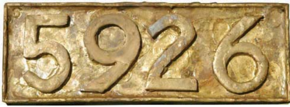
FIGURE 20-3 Brazing used to cover a mild steel house number to both protect it and give it a rustic brass look. Larry Jeffus
