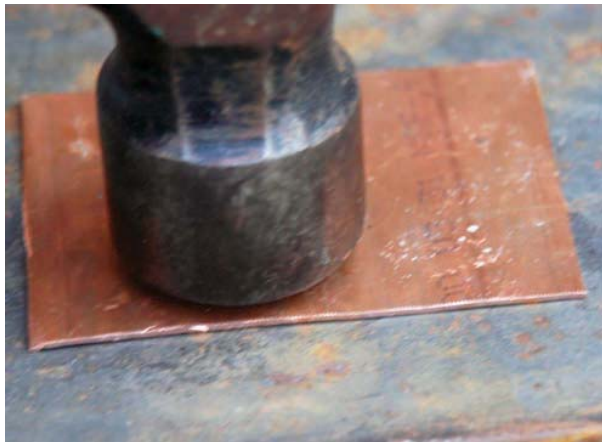
FIGURE 20-27D Flatten the copper. Larry Jeffus
