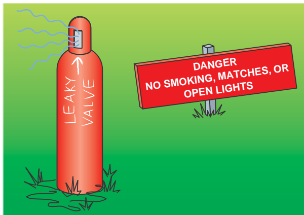
FIGURE 17-40 Identify any cylinder that has a problem by marking it. Larry Jeffus
