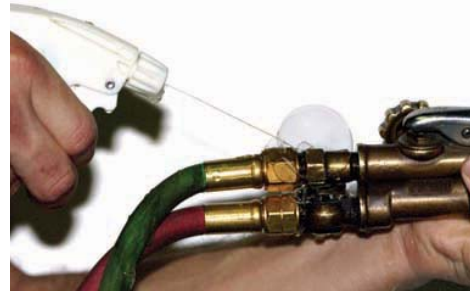
FIGURE 21-14 Leak-check all gas fittings. Larry Jeffus
