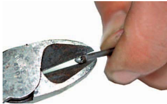
FIGURE 15-32 Using wire cutters to correctly break the tungsten. Larry Jeffus
