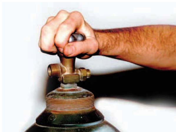
FIGURE 17-28 Cracking the oxygen and fuel cylinder valves to blow out any dirt lodged in the valves. Larry Jeffus
