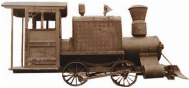
FIGURE 1-2C Riveted narrow-gauge logging train, once used along the coast of the Olympic Peninsula in Washington State. Larry Jeffus
