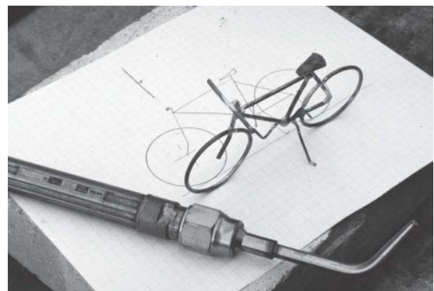
FIGURE 20-49 Be careful not to overheat the joints so that the braze metal does not run. Larry Jeffus
