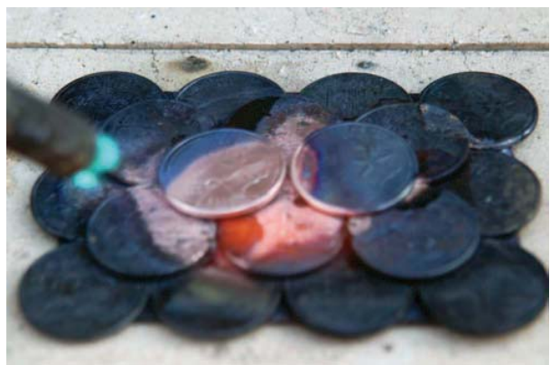
FIGURE 20-35 Angle the torch so that the new coins and the previously brazed coins heat uniformly. Larry Jeffus
