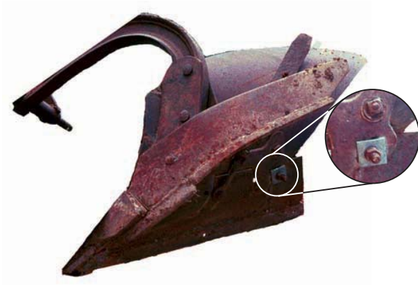
FIGURE 21-92 Nuts and bolts on this rusty plow could not be taken off without a torch. Larry Jeffus
