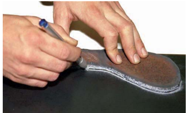
FIGURE 1-4 One way to lay out parts, is to trace them. Larry Jeffus
