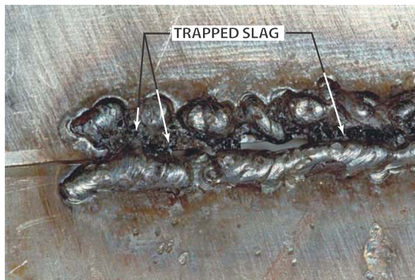
FIGURE 9-43 Moving the electrode from side to side too quickly can result in slag being trapped between the plates. Larry Jeffus
