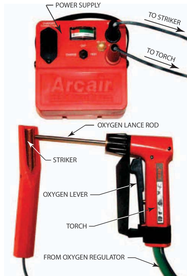
FIGURE 23-13 Arcair SLICE portable cutting system that uses sparks created between the striker and tube to ignite the oxygen lance rod for cutting. Larry Jeffus
