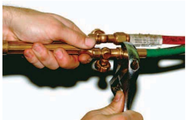
FIGURE 17-14 One hose fitting will protect the threads when the other nut is loosened or tightened. Larry Jeffus
