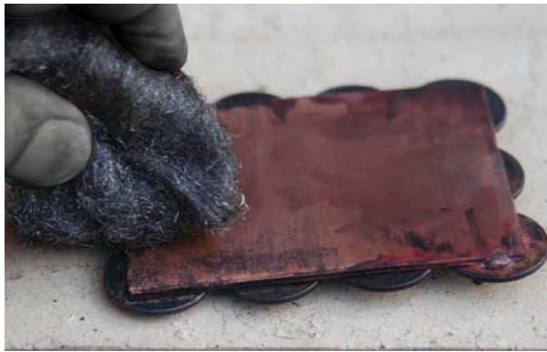
FIGURE 20-36 Use steel wool or a sand cloth to clean off the oxides. Larry Jeffus
