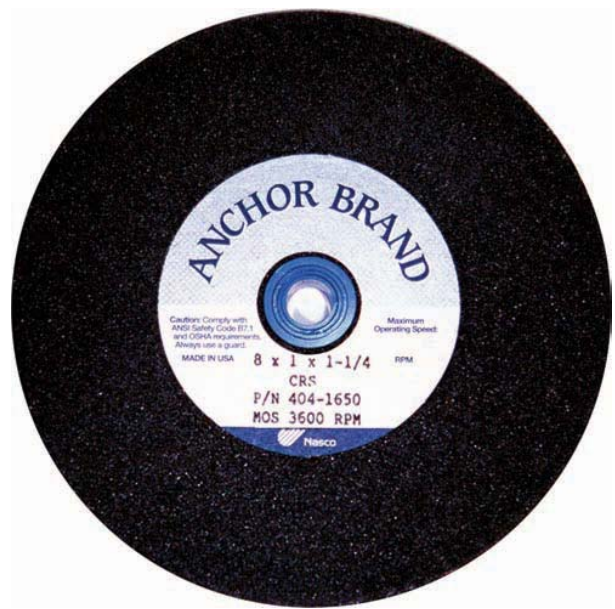
FIGURE 2-48 Always check to be sure that the grinding stone and the grinder are compatible before installing a stone. Larry Jeffus
