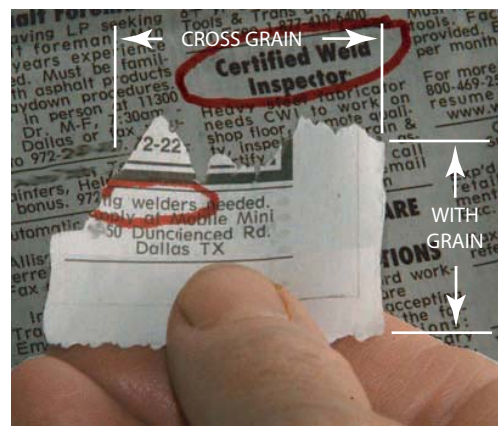
FIGURE 6-8 (A) A metal's strength is affected by the direction it is rolled because of its grain structure. (B) The effect of grain structure can be seen on a newspaper as it is torn. Larry Jeffus
