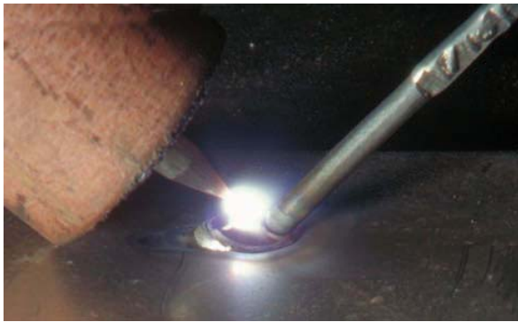
FIGURE 16-29A Establish a molten weld pool and dip the filler rod into it. Larry Jeffus
