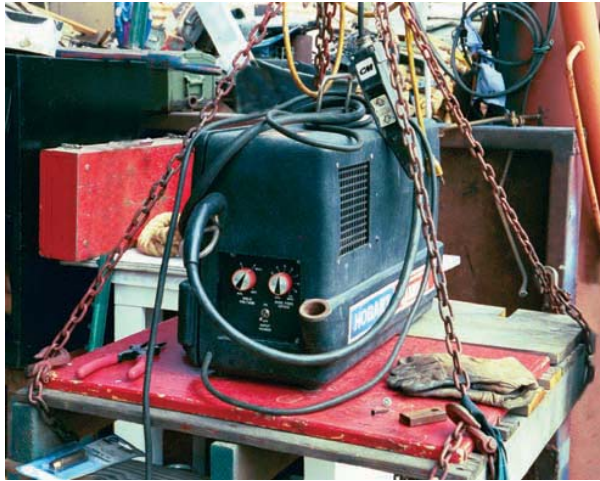
FIGURE 13-2 FCA welder sitting on a wood frame so that it can be lifted closer to the welding. Larry Jeffus
