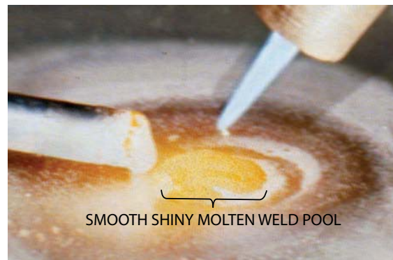
FIGURE 18-7 Neutral flame (balanced oxygen and acetylene). Larry Jeffus
