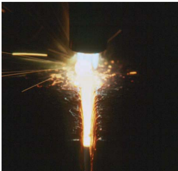
FIGURE 21-56 Watching both the torch track and the stream of sparks from the bottom of the cut will help you adjust your cutting speed. Larry Jeffus
