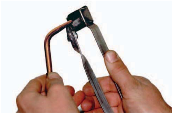
FIGURE 17-42 Spark lighter held too close over the end of the tip. Larry Jeffus
