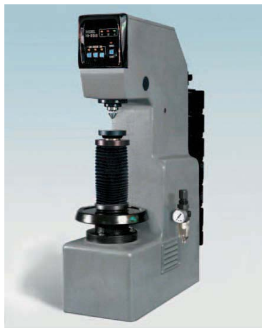
FIGURE 30-42 Brinell hardness tester. Newage Testing Instruments, an AMETEK Co.
