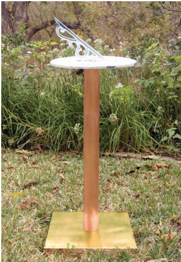
FIGURE 20-4 Sanded and polished braze metal covering a steel base plate. Larry Jeffus
