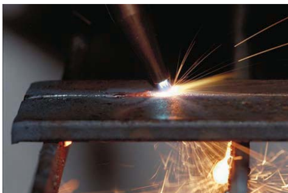
FIGURE 21-34 A good cut showing a steady stream of sparks flying out from the bottom of the cut. Larry Jeffus
