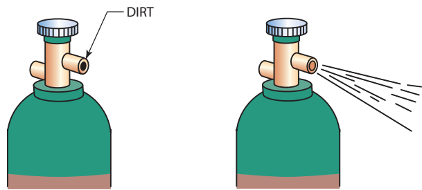
FIGURE 16-8 During transportation or storage, dirt may collect in the valve. Cracking the valve is the best way to remove any dirt. Larry Jeffus
