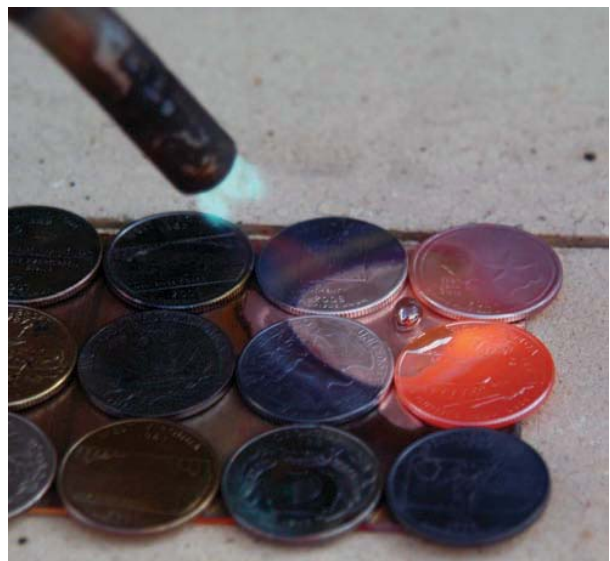
FIGURE 20-31 Watch to see that you do not overheat the coins. Larry Jeffus
