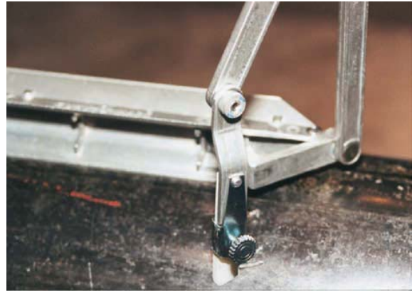
FIGURE 21-88 Hold the base securely so that the arm can be swung around the pipe. Larry Jeffus
