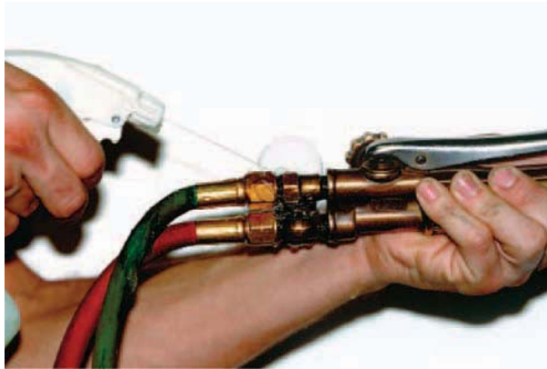
FIGURE 17-39 Spray fittings with a leak-detecting solution. Larry Jeffus
