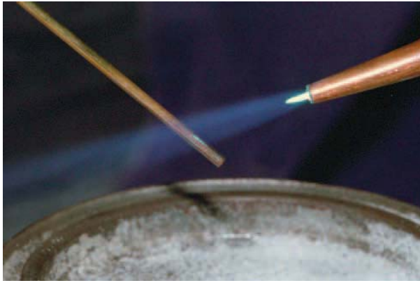
FIGURE 19-30A Heating a brazing rod. Larry Jeffus
