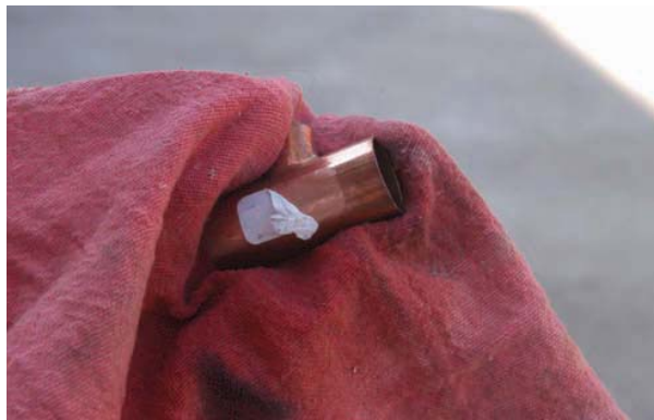
FIGURE 20-53 Use a solvent to remove any sticker adhesive that might remain. Larry Jeffus
