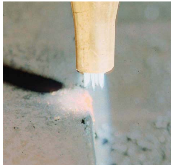
FIGURE 21-48 Starting a cut on the edge of a plate. Notice how the torch is pointed at a slight angle away from the edge. Larry Jeffus
