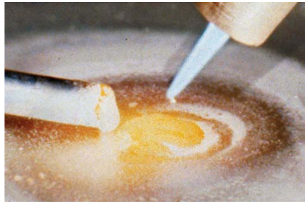
FIGURE 18-28 Adding filler metal to the leading edge of the molten weld pool. Larry Jeffus
