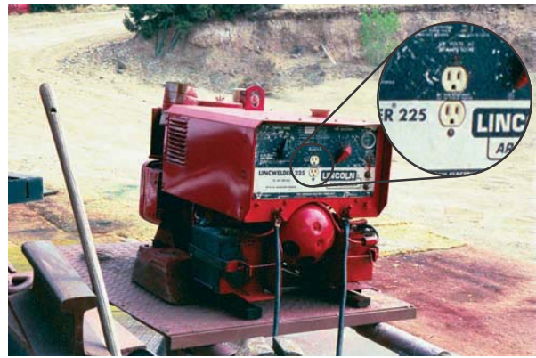
FIGURE 22-3 Portable welder's auxiliary power plug can be used for plasma cutting. Larry Jeffus
