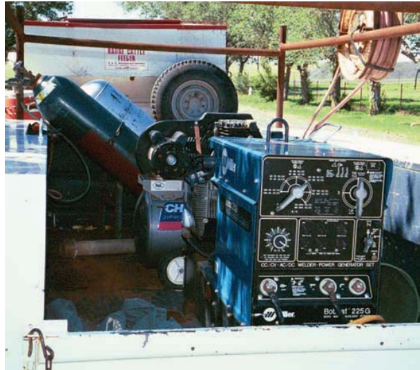
FIGURE 2-56 Secure oxygen and fuel cylinders on vehicles. Remove regulators and replace cylinder valve safety caps any time the vehicle is in motion. Larry Jeffus
