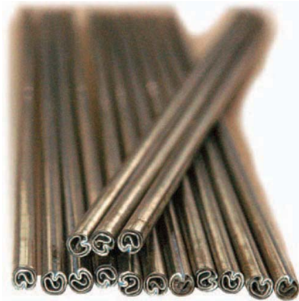
FIGURE 23-12 Oxygen lance rods may be rolled out of flat strips of special alloys to form a tube. Larry Jeffus
