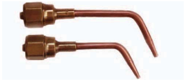
FIGURE 17-16 A variety of tip styles and sizes for one torch body. Larry Jeffus
