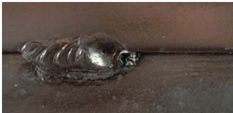
FIGURE 9-39 The tack weld should be small and uniform to minimize its effect on the final weld. Larry Jeffus
