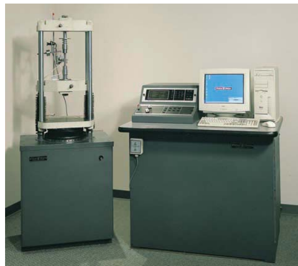
FIGURE 30-21 Typical tensile tester used for measuring the strength of welds (60,000-lb universal testing machines). American Welding Society
