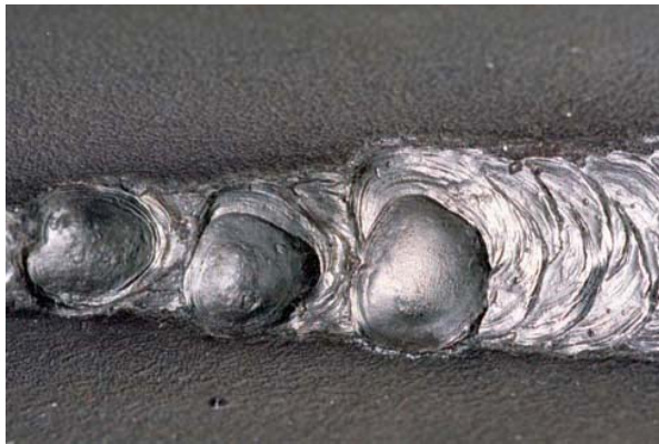
FIGURE 12-61 Each of the welds on the large multi-pass fillet weld on the anvil needs to be made all the way to the end of the joint and not stopped short of the end. Larry Jeffus
