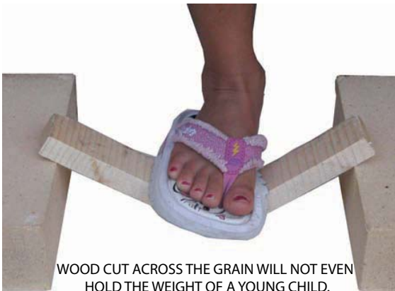
FIGURE 21-76 Metal, like wood, is stronger with the grain than it is across the grain. Larry Jeffus
