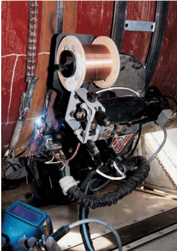
FIGURE 25-9 Automatic GTA machine welding along the seam of a stationary pipe. The Lincoln Electric Company
