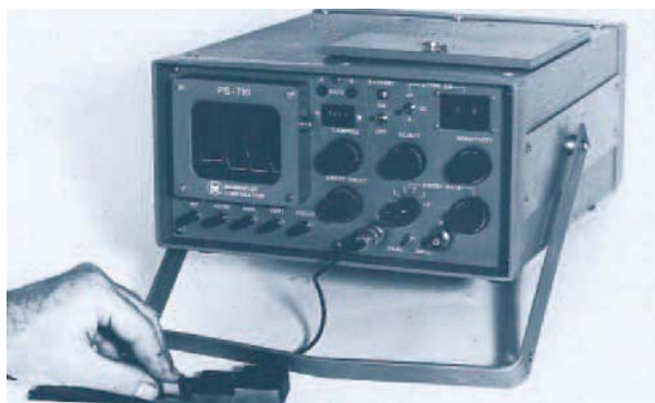
FIGURE 30-39 Portable ultrasonic inspection unit. Magnaflux, A Division of ITW
