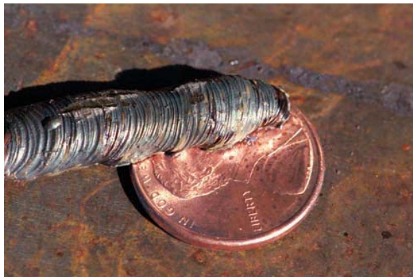
FIGURE 28-1 Improper welding technique for filler metal resulting in lack of fusion. Larry Jeffus
