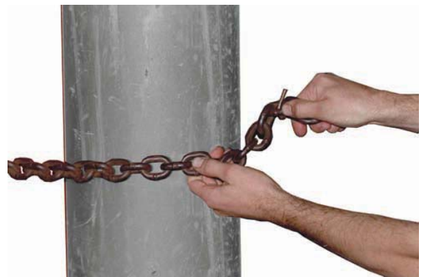
FIGURE 11-33 Make sure the gas cylinder is chained securely in place before removing the safety cap.
