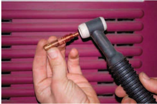
FIGURE 15-42 Inserting collet and collet body. Larry Jeffus
