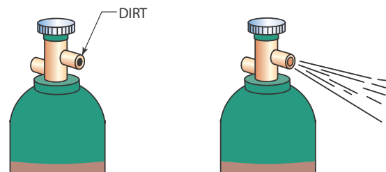
FIGURE 15-37 During transportation or storage, dirt may collect in the valve. Cracking the valve is the best way to remove any dirt. © Cengage Learning 2012
