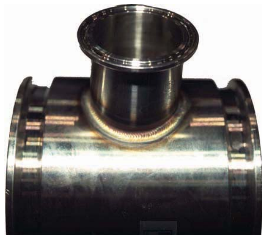
FIGURE 1-7 Gas tungsten arc welding was used to join this stainless steel flange to pipe. Larry Jeffus
