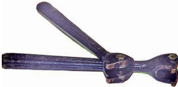
FIGURE 2-50 Use a grinding stone redressing tool as needed to keep the stone in balance. Larry Jeffus
