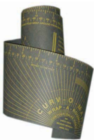
FIGURE 10-43 Wrap-A-Round used to lay out pipe. Larry Jeffus
