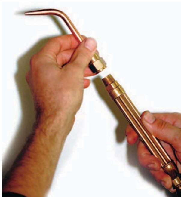
FIGURE 17-33 Select the proper tip or nozzle and install it on the torch body. Larry Jeffus
