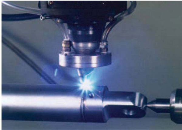
FIGURE 24-7 Gas filter, laser welded. Preco, Inc.
