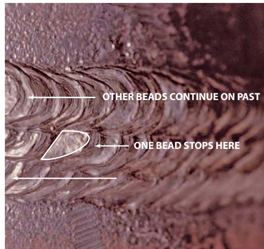
FIGURE 10-20 Avoid starting and stopping all weld passes in the same area. Larry Jeffus
