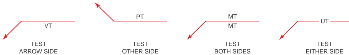
FIGURE 5-35 Testing symbol used to indicate the side that is to be tested. American Welding Society
