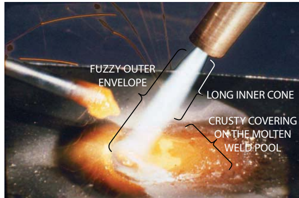
FIGURE 18-6 Carbonizing flame (excessive acetylene). Larry Jeffus
