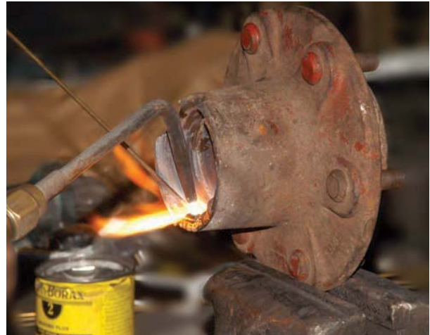
FIGURE 20-5 Braze metal used to repair a worn wheel bearing race. Larry Jeffus
