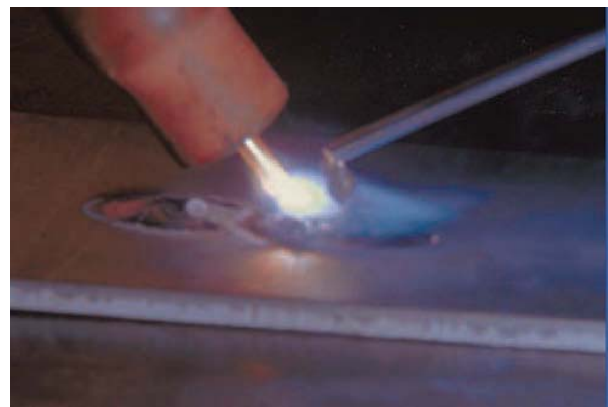
FIGURE 16-4 Filler rod being melted before it is added to the molten pool. Larry Jeffus
