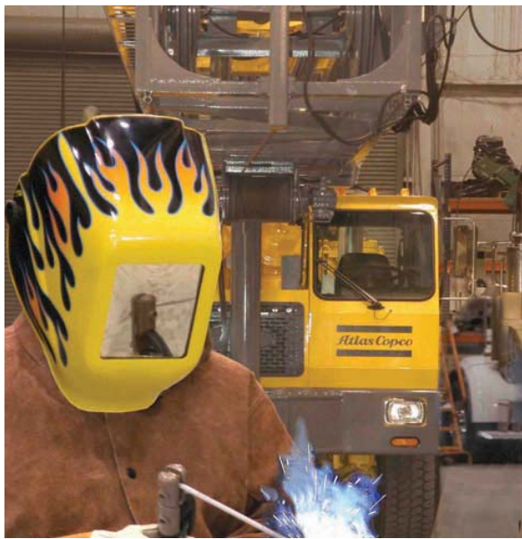
FIGURE 2-7 Typical arc welding helmets used to provide eye and face protection during welding. Larry Jeffus
