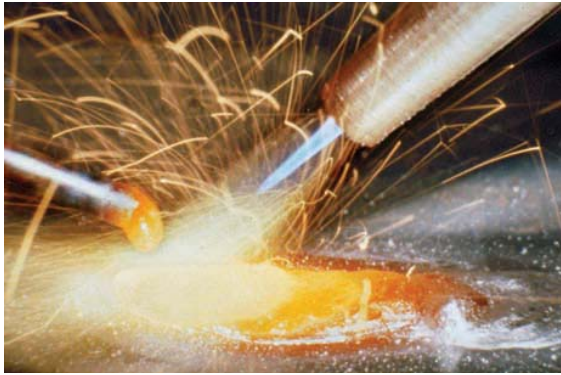
FIGURE 18-8 Oxidizing flame (excessive oxygen). Larry Jeffus
