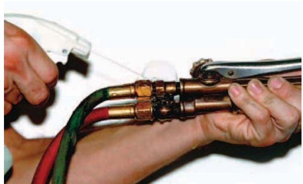
FIGURE 17-15 The torch valves should be checked for leaks, and the valve packing nut should be tightened if necessary. Larry Jeffus
