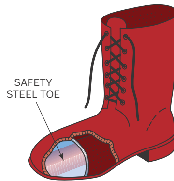
FIGURE 2-24 Safety boots with steel toes are required by many welding shops. © Cengage Learning 2012
