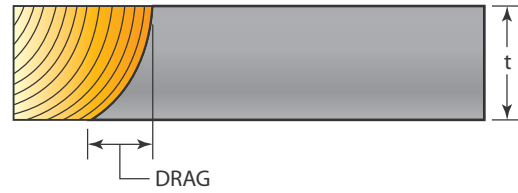
FIGURE 21-41 Drag is the distance by which the bottom of the cut lags behind the top. © Cengage Learning 2012
