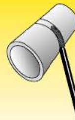
Pipe fixed horizontal axis, welding downhill: PJ/5G
