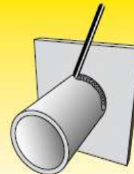
Pipe fixed horizontal axis, welding uphill: PH/5F
