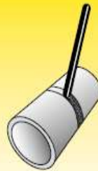
Pipe fixed horizontal axis, welding uphill: PH/5G
