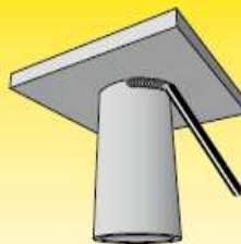
Pipe fixed vertical axis, welding overhead: PD/4F
