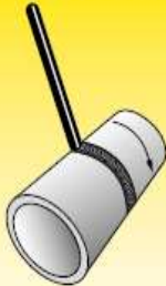
Pipe rotates horizontal axis Downhand: PA/1G
