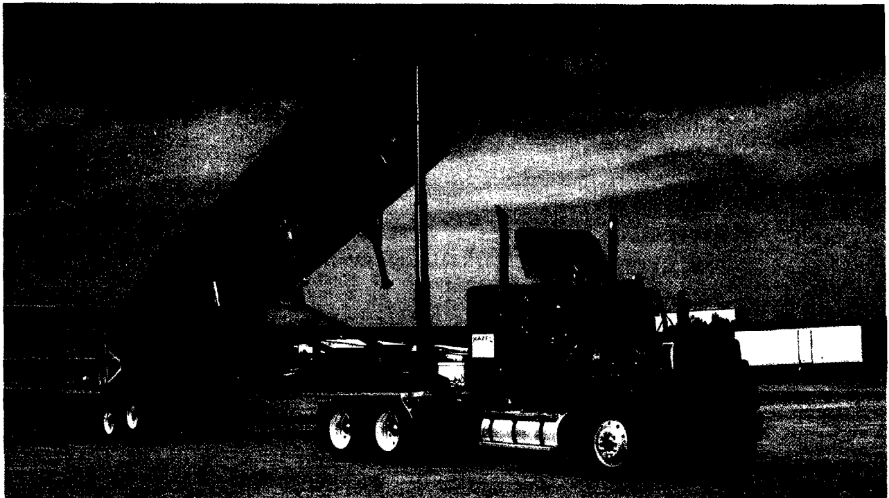
Figure 1.48—Aluminum Dump Trailer made from 5454-H34 Sheet, 6061-T6 Extrusions, and Gas Metal Arc Welded with 5556 Filler Metal
