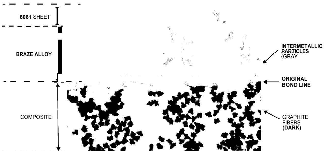
Figure 7.36—Brazed Interface Between 6061 Sheet and Al-7Zn/C with 718 as Braze Alloy (x500)
