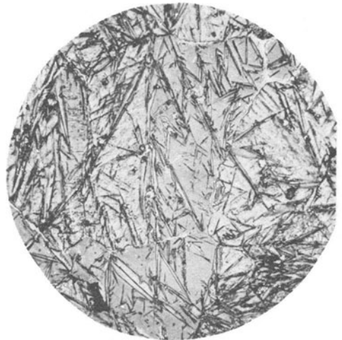
Fig. 4.10 — Quenched martensite (500 X, before reduction, etched) showing acicular structure.
