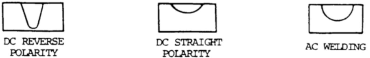
Figure 5-38. Comparison of penetration contours.
