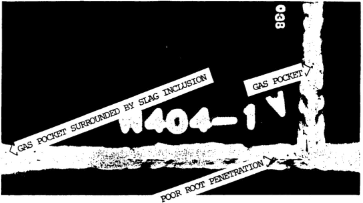
Figure 13-8. Internal weld defects disclosed by X-ray inspection.
