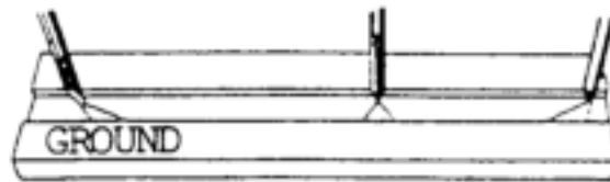
Figure 6-61. Effect of ground location magnetic arc blow.
