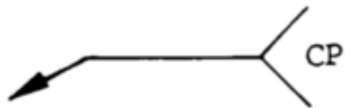
Figure 3-22. Complete penetration indication.
