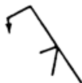
Figure 3-18. Construction of symbols, perpendicular leg always to the left.
