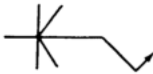
Figure 3-19. Construction of symbols, arrow break toward chamfered member.
