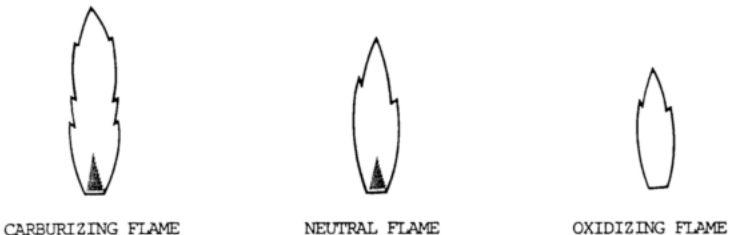
Figure 11-3. What MAPP gas flames should look like.
