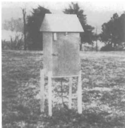
Figure 19-1. High-volume sampler.
