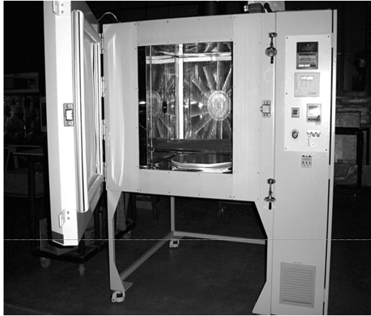
Figure 10.6 A high-performance stress screening chamber ( photo courtesy of G. Martell and G. Korosi. )
