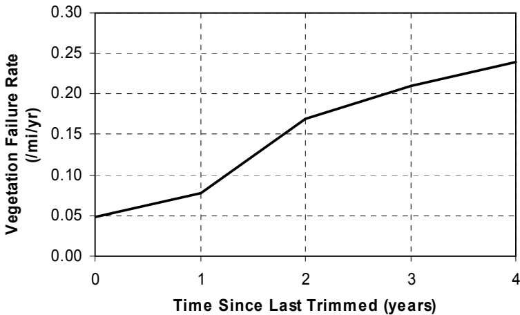
Figure 6.20. Tree trimming cycle time can have a profound impact on vegetation-related failure rates on overhead lines. The above data, obtained from a utility in the midwestern US, 20 shows that vegetation-related failures increase by nearly a factor of five from the time a right-of-way is trimmed through four years without additional trimming.
