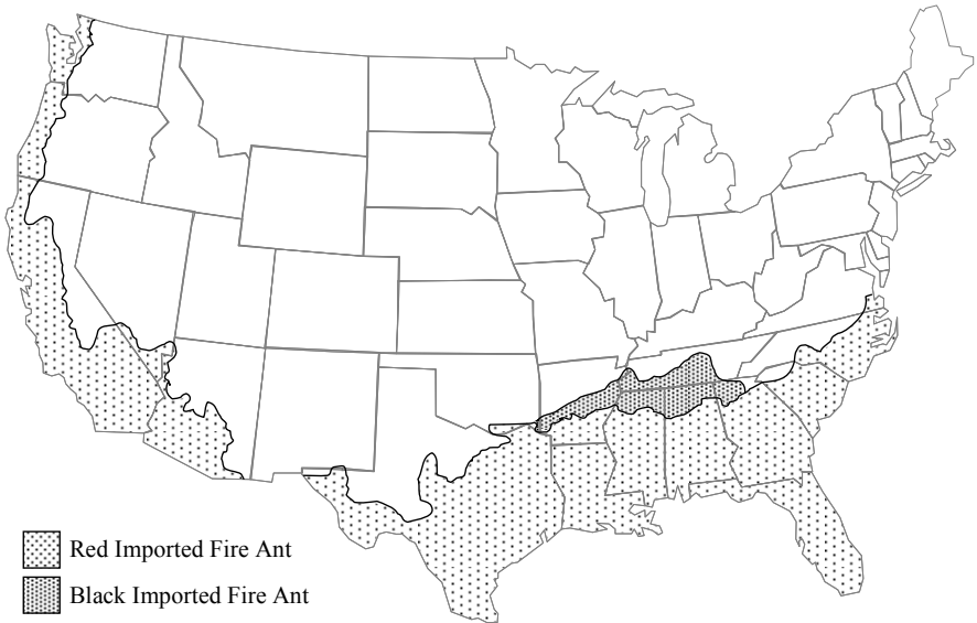
Figure 3.10. Likely areas of future fire ant infestation. Fire ants were accidentally introduced into the US from South America in the early 1900s. Since then, they have spread widely across the southern US, displacing native ant species and causing reliability problems by building nests in electrical equipment.
