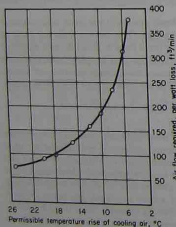
FIG. 6-6 Airflow requirements for limiting temperature rise in transformer vaults. (From EEI Underground Systems Reference Book .)
