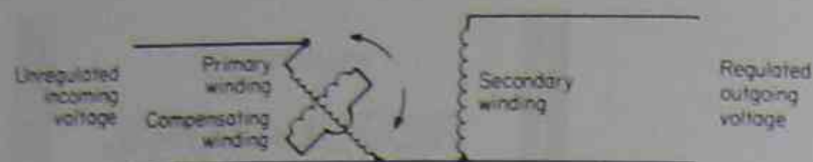
FIG. 12-1 Induction regulator windings.
