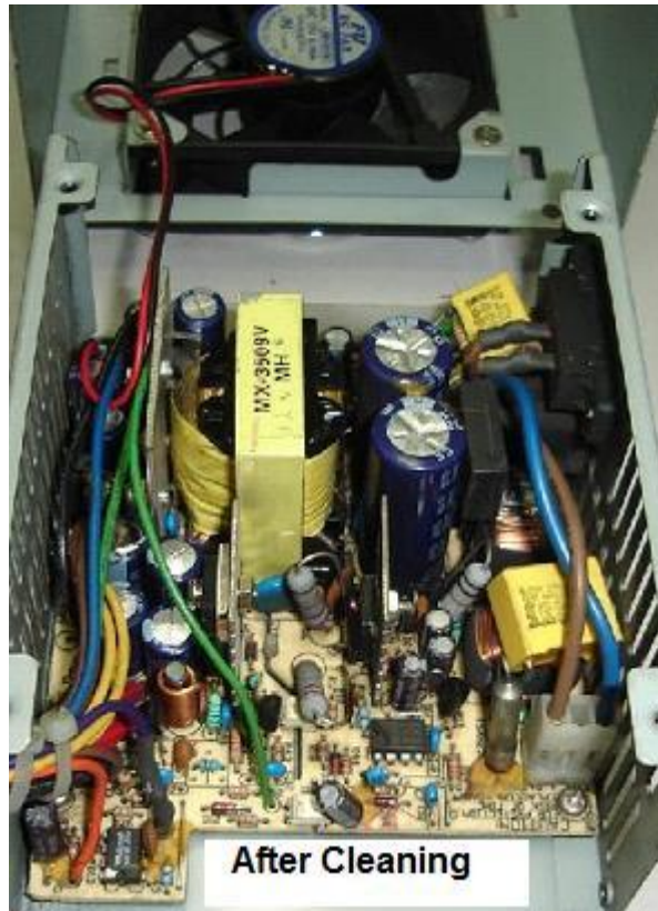
Figure 20.7- After Cleaning With A Vacuum Cleaner And A Brush
