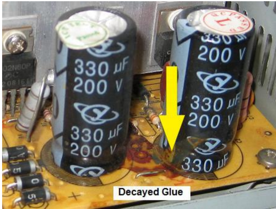
Figure 20.4- Decayed Glue Found In ATX Power Supplies
