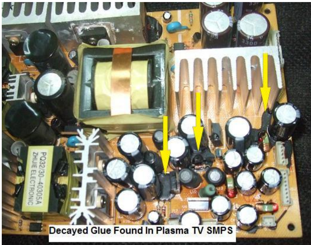
Figure 15.12- Decayed Glue Found In Circuit Board
