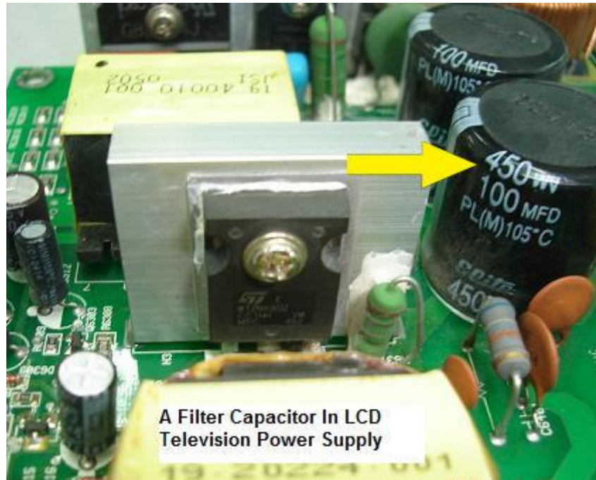
Figure 10.1- Filter Capacitors In LCD Television SMPS
