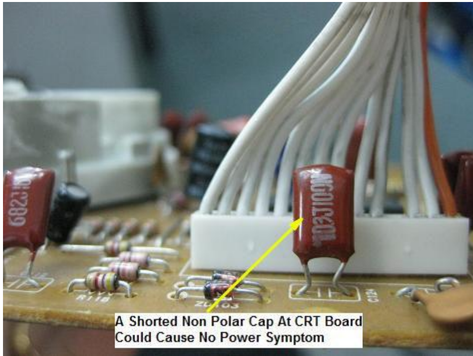
Figure 18.1- Shorted Non Polar Capacitor At CRT Board
