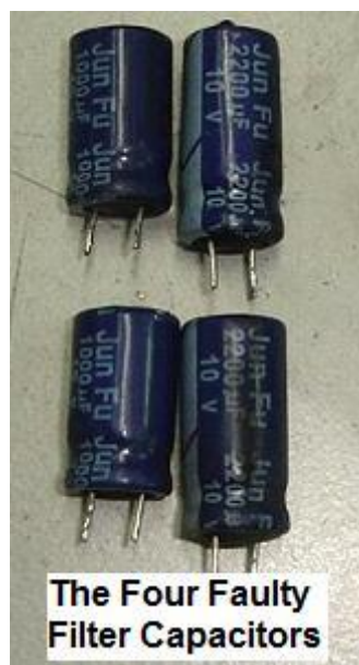
Figure 20.8- The Four Faulty Filter Capacitors
