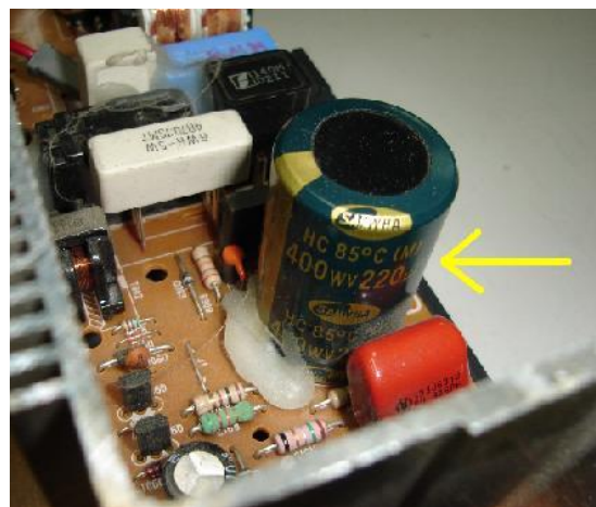
Figure 10.2- A Large Filter Capacitor In CRT Monitor Power Supply Section
