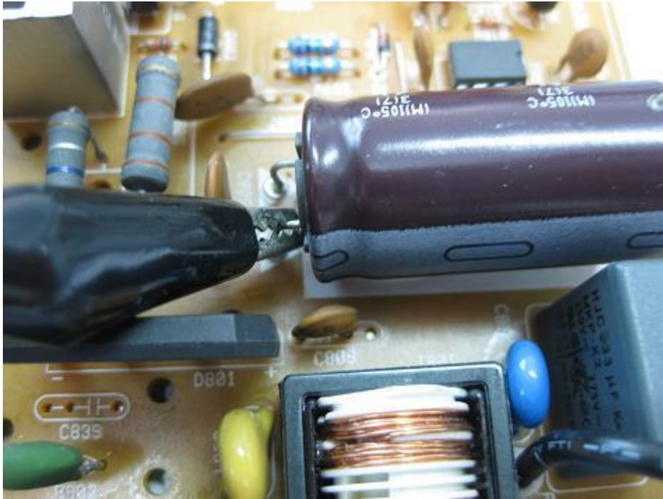
Figure 12.3- Connecting The Oscilloscope Ground Lead To The Negative Side Of Filter Capacitor In Primary Side
