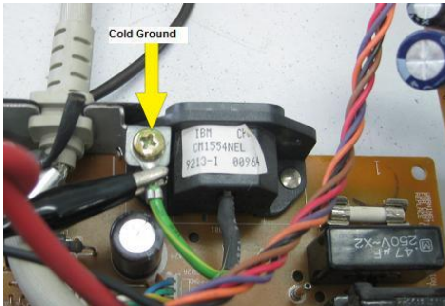
Figure 12.4- Connect The Scope Ground To Cold Ground If You Want To Check The Secondary Side
