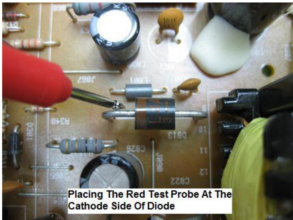
Figure 11.9- The Right Way To Place The Red Probe To Check Positive Output Voltage Of SMPS
