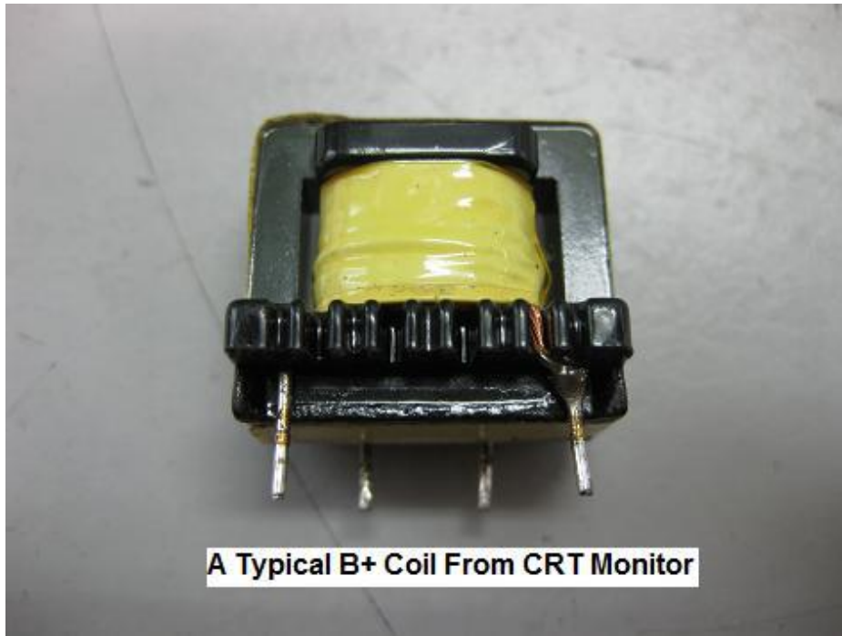
Figure 14.9- A Typical B+ Coil From CRT Monitor
