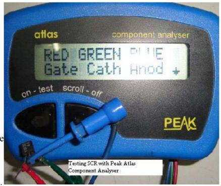
The tester will begin to analyze the SCR and prompt you with the display such as "Sensitive or low power thyristor" before it tells you the exact pin outs of G, A and C. After the first test, the tester will eventually show you
