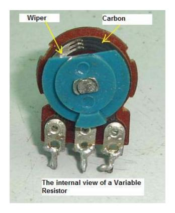
Failure among variable resistors usually takes form of intermittent connections between the wiper blade and resistive film. Sometimes it also can be burnt due to overload of currents and develop an open circuit. Remember that film slowly wears away as the wiper moves back and forth across it. After sometimes the overall film can wear away that which the wiper cannot make a good contact at certain points. The poor contact can cause all types of erratic or intermittent operation.
