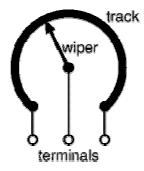
Internal view of Variable resistor
