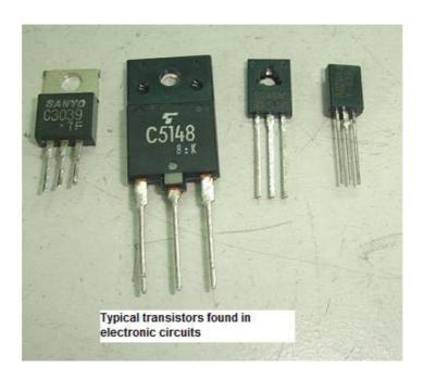
Transistors are solid –state devices similar in some way to the diodes you have studied. Transistors are more complex and can be used in many more ways. They are very important and can be found in almost all modern electronic equipment. The name transistor is derived from "trans resistor", meaning that it **changes resistance**. Unlike a diode, a transistor has three leads. The three transistor leads are designated as **Base (B)**, **Collector (C)**, and **Emitter (E)**.
