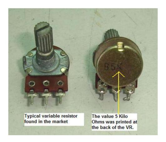
Variable resistors also called potentiometers or rheostats, employ a movable metal blade resting along a ring of resistive film. You can change the resistance by turning the knob.
