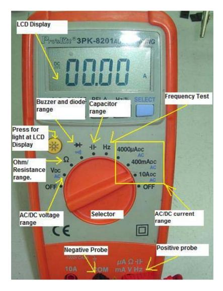
Black test lead plugs into meter terminal marked Common, Com,or  $\bigcirc$  Red test lead plugs into meter terminal marked  $\bigcirc$   $\bigcirc$   $V-\Omega-mA$ .
