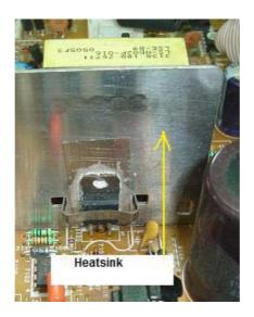
The heat generated by current flowing between the collector and emitter junctions of a transistor causes its temperature to rise. This heat must be conducted away from the transistor otherwise the temperature rise may be high enough to irreparably damage the P-N junctions inside the transistor. Power transistors produce a lot of heat, and are therefore usually mounted to a piece of aluminium with fins, called a heat sink.
