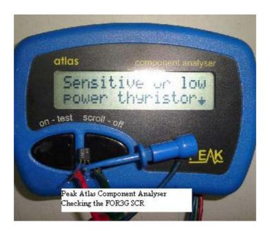
Once you know the pin outs of the G, A and C legs you can begin to test the SCR. If you have the Peak electronic atlas component analyzer tester, what you need to do is to connect the three small clips to each pin of the SCR (any part number will do).
