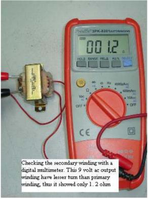
Perform a ringing test with a ringer tester like using the dick smith coil tester. Checking the ohms resistance or continuity on a linear transformer is not accurate as compared when using a ringer tester. However there is still one disadvantage which is the winding can go shorted when under
