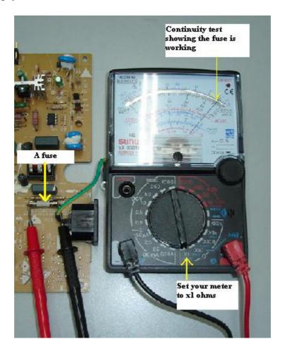
Measuring a fuse on board with an analogue multimeter
