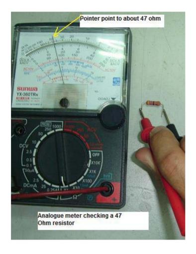
If you get more than 47 ohm say 150 ohm, this mean that the resistor has gone up in resistance and need replacement. If it doesn't show any reaction after putting the probes across the two points of the resistor, then we can conclude that the resistor has open circuit (bad). Remember to press a little bit hard on the leads of the resistor while measuring it otherwise you may not get a precise reading or intermittent reading could occur.
