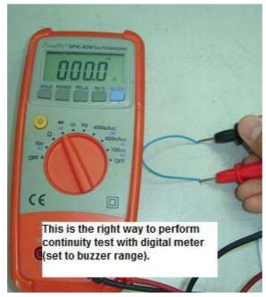
You can also use a digital meter that have the buzzer sound to test the connection. If you heard the buzzer sound while measuring the wire or connection, this means that the connection or internal wire is good.
