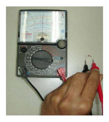
Use analogue multimeter to test zener diode
