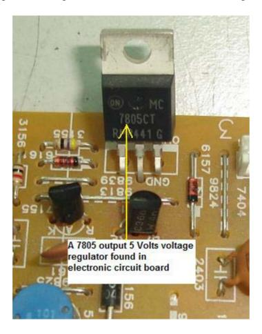
For your information the input voltage must have at least two volts higher than the input voltage. That's mean if you want to get a 12 V output from a 7812 voltage regulator, the input voltage have to be at least 14 V and above. Don't expect to use a 5 V dc input to produce 12 V output, this way won't work!
