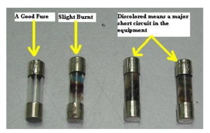
A blown fuse can indicate how severe the short circuit is.
