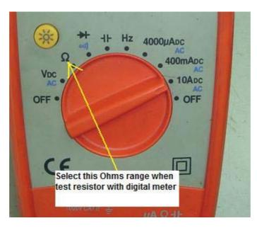
Personally I do not use analogue meter to test resistor as the result shown on the meter panel only makes you have to guess what the resistor value is. You may ask yourself, is it 47 ohm or 47.5 ohm or even 47.7 ohm? By using digital meter the LCD display in your meter will show you the exact value of the resistance under test. It is more accurate than using analogue meter.
