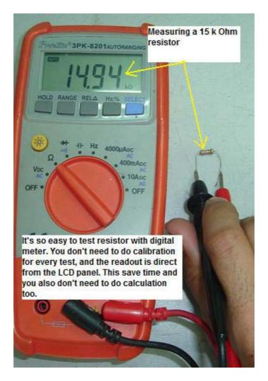
First, select the Ohm range and place your test probes across the two points of the resistor as shown in the photo. **Digital meter does not need any calibration compare to analogue meter** where you have to adjust the adjuster to make it zero Ohm before you begin to do measurement. The result shown at the LCD display of the digital meter is the exact resistance value of the resistor.
