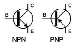
Fig 1: The circuit symbols for the two transistor types a) NPN b) PNP
