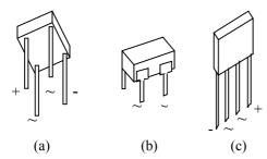
Fig 1: Some examples of bridge rectifier
