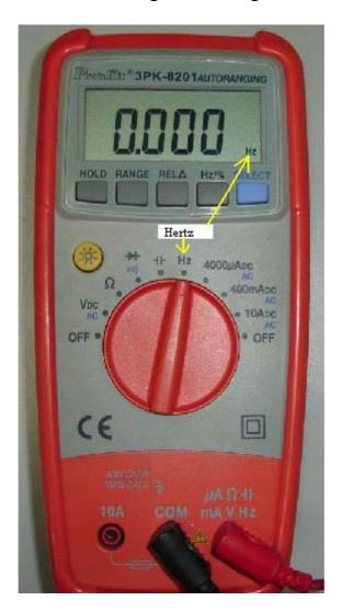
Frequency counter in a digital multimeter
