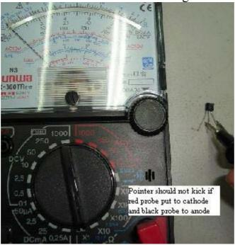
Make sure set to X1 ohms to test SCR
