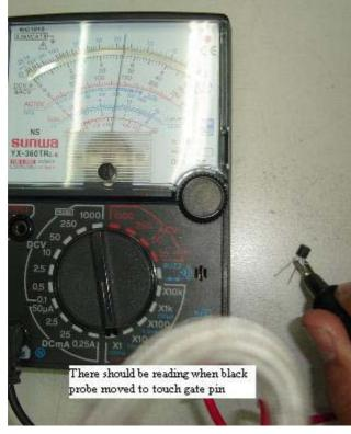
Removing the black probe from the GATE pin (the black probe still touching the Anode pin) you would noticed that the resistance continues to be there (low resistance). This is due to the conduction of SCR as the meter battery is usually able to supply current more than the holding current.
