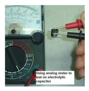
If it still don't flick then the capacitor under test have developed an open circuit. This is a rather old method to test capacitors because even though a capacitor can charge and discharge, **this does not mean the capacitor value is good.** Due to this problem, digital capacitance meter was developed.
