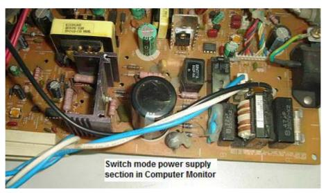
Switch Mode Power Transformer (SMPT) are used in switch mode power supplies in electronic equipment such as Computer Monitor, TV, DVD and etc. The function of SMPT is to convert the AC wave to some other value, lower or higher. The input is called primary winding while the outputs are secondary windings.
