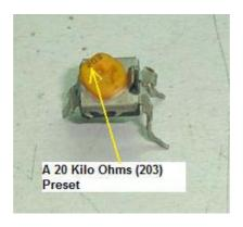
These are miniature versions of the standard variable resistor. They are designed to be mounted directly onto the circuit board and tuned only when the circuit is built. For example to set the colours of Computer Monitor by turning the preset in the Cathode Ray Tube (CRT) board.
