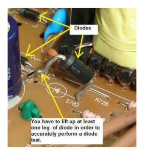
To be absolutely sure, you will need to lift, or disconnect, one diode lead from the circuit to avoid back circuits. Unless you are very sure about the board you are checking. Sometimes I do found bad diodes when checking it on board. Your experienced will tell you when to test a diode on-board or off-board. If you are a beginner, I highly suggest that you measure a diode with a lead removed from the board to avoid any confusion results from your meter.
