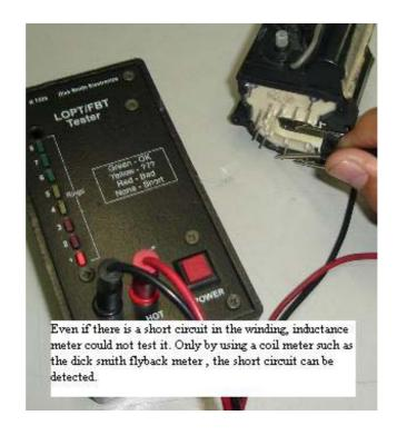
Using Flyback Tester To Test Flyback Transformer
