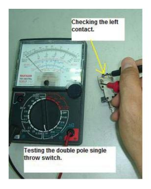
Some switches have dual on/off contact and is called double pole single throw switch (DPST). A DPST switch is often used to switch mains electricity because it can isolate both the live and neutral connections. Testing the DPST switch is relatively simple, test the contact at one time before you test on the other contact. Testing method is the same just as when you are testing the single on/off switch above. Look at the photos and should understand what I meant.
