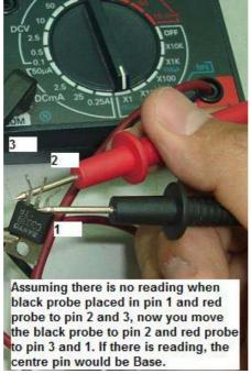
The diagram in Figure 2 assumes you are testing an unknown type of transistor. Set your meter to the lowest ohm's range i.e.  $\mathbf{Rx}\mathbf{1}\Omega$ . From the six combination of test result you will know the transistor is belonging to which type.
