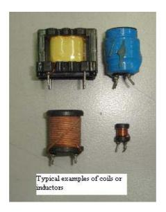
Testing coil is very easy compares to checking three leads components such as SCR, FET and etc. In general, a coil consists of many turns or wire wrapped around a common core. The core could be made of iron or even air. It is label as "L" on circuit board.
