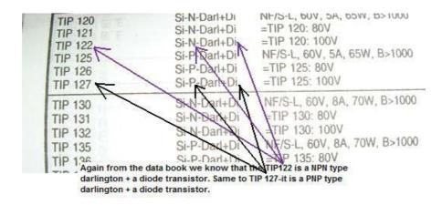
Because of the built in diode, the result that you get is completely different from testing the Darlington transistor that have no diode built into it. It is difficult to find the Base, Collector and the Emitter pins due to the built in diode. I guess you have to refer to semiconductor data books or even the internet to look for its pin outs.
