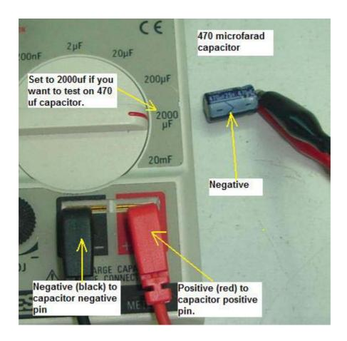
Testing electrolytic capacitor with digital capacitance meter
