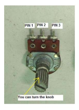
If you measure pin 1 and 3 you will get the variable resistor Ohms reading. Now use either one probe to touch pin 1 and 2 (Fig a) of variable
