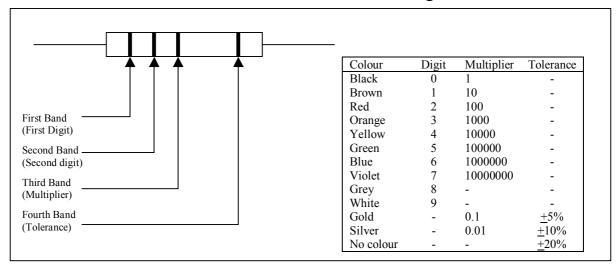
TABLE 1- Showing four colours band of resistor and their meanings.
