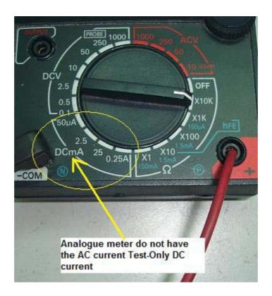
In most electronic troubleshooting and repair, you will rarely take current measurements. Most general purpose digital multimeters allow you to measure AC current (ACA or Iac) and DC current (DCA or Idc) in a circuit, although there are often few ranges to choose from. **Normally analogue meter do not have the AC current range.**
