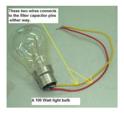
A 100 watt bulb use to discharge filter capacitor
