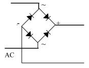
Fig 2: Schematic for diodes wired as a full-wave bridge rectifier
