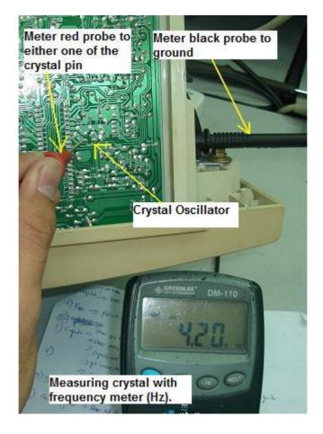
The right way to test crystal oscillator in electronic equipment
