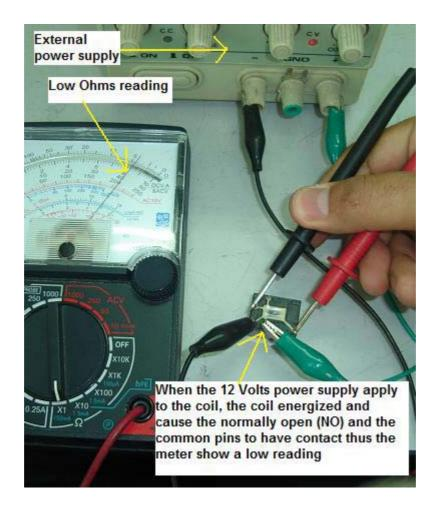
If you place your analogue meter probes set to X 1 Ohm across the "common (Com)" and the "normally close (NC)" pin and when you hear the "tic" sound, you will see that the meter pointer will drop from the zero Ohm to infinity (indicating open circuit).
