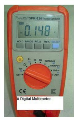
Multimeters (analogue and digital) are one way in which you can "see" what's going on in an electrical circuit. Voltmeters, ohmmeters, and ammeter are essential in all electric work. Multimeters can go by many
