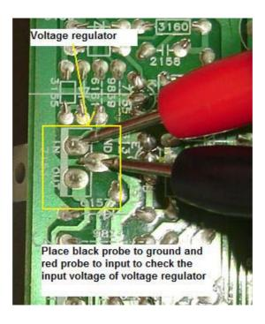
Place the red probe to out and you can test the output voltage
