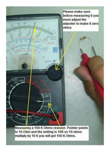
In order to check a 100 K ohm resistor you have to select the X 10 K Ohm range. Follow the procedure explained above and you should be able to get the measurement.
