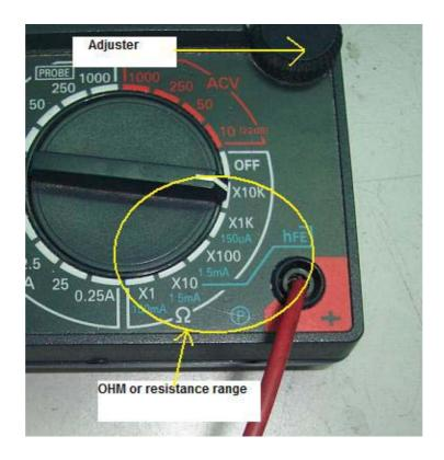
First you must know the resistor value before you take any measurement. With the resistor colour band calculation you have read from the previous section, I'm sure you have no problem in identifying resistor value by looking at the colour bands. Assuming you are measuring a resistor with the colours of "yellow, purple, black and gold", from calculation it is a 47 Ohms resistor with 5 % tolerance.
