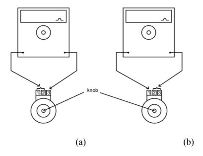
Fig 1: Testing a variable resistor with a analogue multimeter
