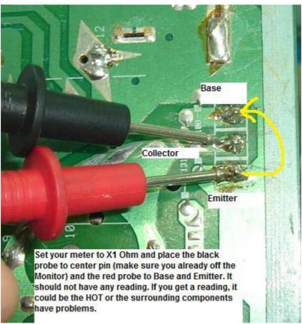
It is very easy to check on board if the HOT is shorted or not. Using your analogue meter set to X 1 Ohm and place the back probe to centre
