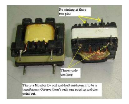
Coil or inductor can be test using an analogue, inductance or a coil meter such as the dick smith flyback tester. A coil that is small in size, **I would usually just test it with analogue meter** and you could check it on board too. Set your analogue meter to X1 ohm and place the probes across the small coil.
