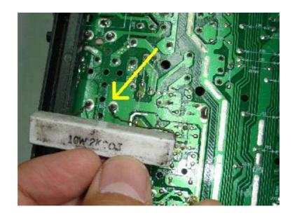
Use a resistor to discharge the capacitor leads
