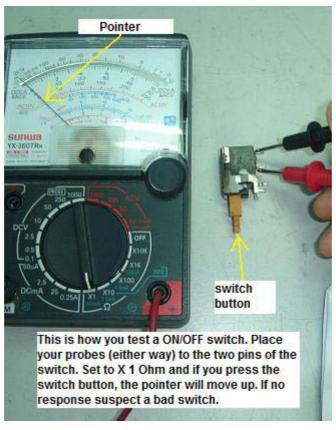
There are many type of switches in the market, some are on/off mechanical switch while some are micro switch. The function of the switch is to act as a contact between two points either to let current flow or to stop it. It is very easy to test switches, just set your meter to X 1 ohm and place your meter test probes to either leg (pin). Now press the switch and you should see the meter's pointer shows zero ohm.
