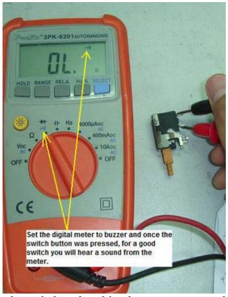
If after pressing the switch and nothing happen, suspect a bad switch. Similarly, you can use a digital meter set to buzzer sound to test a switch. A good switch with a good contact should make the digital meter to produce the buzzer sound. No sound means the switch is defective.
