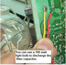
The right way to discharge capacitor with light bulb
