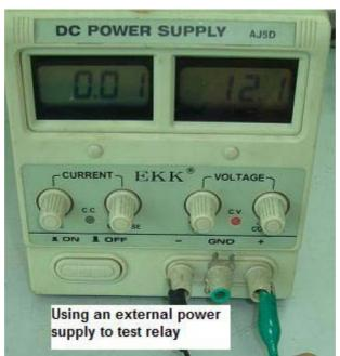
The next step is to connect a power supply across the relay. Use a variable regulated power supply to adjust to the same voltage as what the relay can handle. That's mean; if the relay specification is 5V then you
