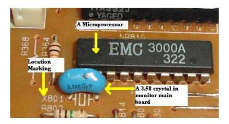
A Crystal and its location marking in a Computer Monitor
