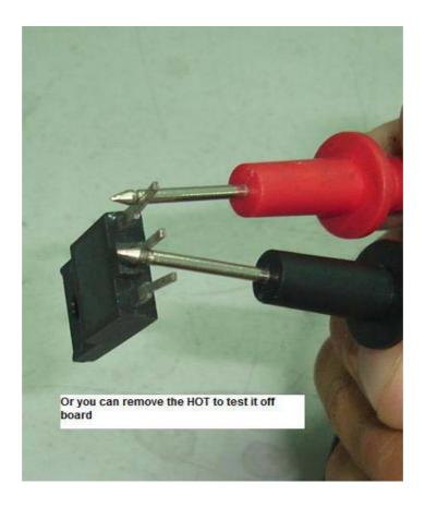
Conclusion- If you measure base (black probe) and collector (red probe) it should have reading.
