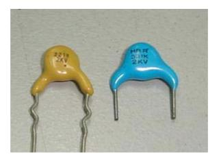
Resin coated ceramic disc capacitors
