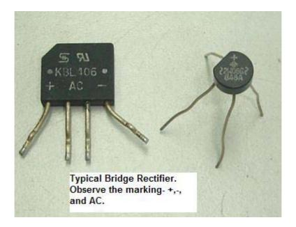
A schematic for the full wave bridge rectifier is drawn in Fig 2. Bridge rectifiers are classified in the same way as single diodes, i.e. by their maximum reverse voltage or Peak Inverse Voltage (PIV) and Forward Current, IF. It is label as "BR" in electronic circuit.
