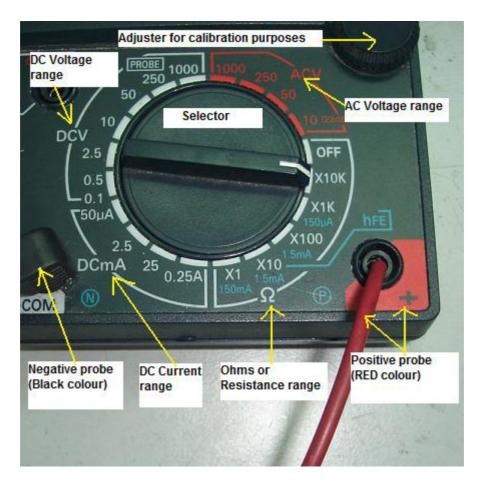
Analogue and digital multimeters have either a rotary selector switch or push buttons to select the appropriate function and range. Some Digital Multimeter (DMMs) are auto ranging; they automatically select the correct range of voltage, resistance, or current when doing a test. However you still need to select the function.
