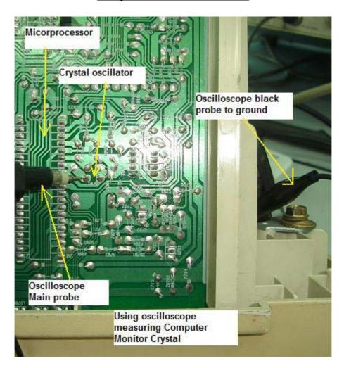
How to measure crystal frequency with oscilloscope
