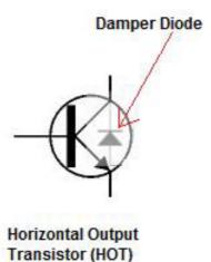
If you are repairing Television and Computer Monitor, I'm sure you had seen a horizontal output transistor (HOT) before. This transistor is use to switch the flyback transformer and prone to become defective due to the stress of dealing with high voltage. A shorted HOT will usually caused no power, low power, power cycling and power to shutdown. The HOT is mainly a NPN transistor.
