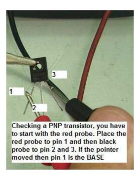
Your test probe placement must be reversed in order to check for PNP type of transistor as shown in Figure 3.
