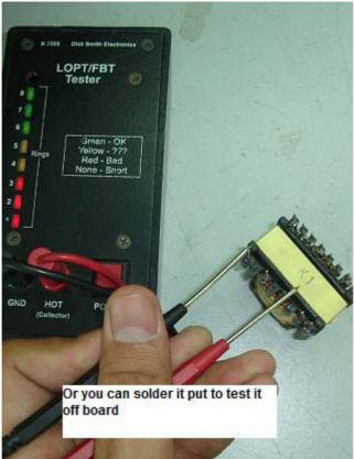
Placing the flyback tester probes to the primary winding of the switch mode power transformers, a good measurement will usually between of 4-8 bars LED lights up. If it indicates only one or two LED bars or the flyback tester LED goes off (no light), this proof that the primary winding have problem. If the primary winding shorted, you can send the SMPT to a rewinding shop for repair.
