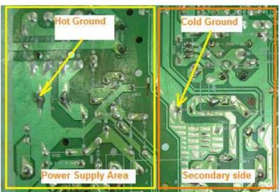
Modern equipment consists of two grounds, one of which is a "hot" ground while the other is a "cold" ground. Hot ground is in the primary side of a switch mode power supply while the cold ground is the equipment ground.
