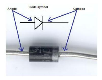
When comes to testing diode, you need a special method to test it. If you do not know how to accurately check a diode, you will not be able to repair or troubleshoot electronic equipment because a spoilt diode you may think that it is good and you will definitely waste your precious time. Diode is label as "D" in circuit board. Usually a rectifier diode can fail in one of the four ways.
