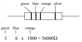
Therefore, the R value is  $56000\Omega$  or  $56k\Omega$  with tolerance  $\pm 10\%$ . (Silver is 10%-please refer back to table 1)
