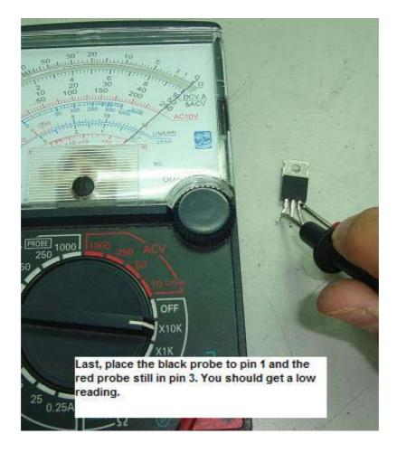
I suggest that you get few of the Darlington transistor from electronic suppliers (with and without built in diode) to play around with it. Record down all the steps you have taken to successfully test this type of transistors before you test on the bad or faulty Darlington transistor.
