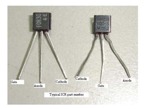
Testing SCR (silicon controlled rectifier) can be done by using an analogue multi meter or specialize tester (such as the Peak electronic atlas component analyzer-http://www.peakelec.co.uk) designed to check semiconductor devices easily. SCR can be found in many electronic circuits. Part numbers such as the FOR3G and MCR 100-6 were very common used in computer monitor.
