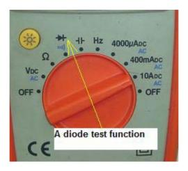
If you don't get any reading either forward or reverse bias, the diode is considered open circuit. The real problem when testing a diode using the diode test function of a digital meter is that an open or leaky diode, the meter sometimes reads okay. This is due to the digital meter diode test output voltage (which you can measure the output test probe using another meter) is around 500my to 2v.
