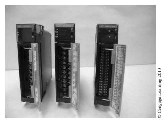
Figure 2-8 AC Input and Output Modules and Analog Input Module
