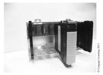
Figure 2–9 Installing a Module in an I/O Rack
