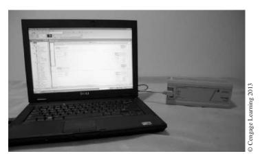
Figure 1–8 Laptop Computer Connected to a AB MicroLogix 1000
