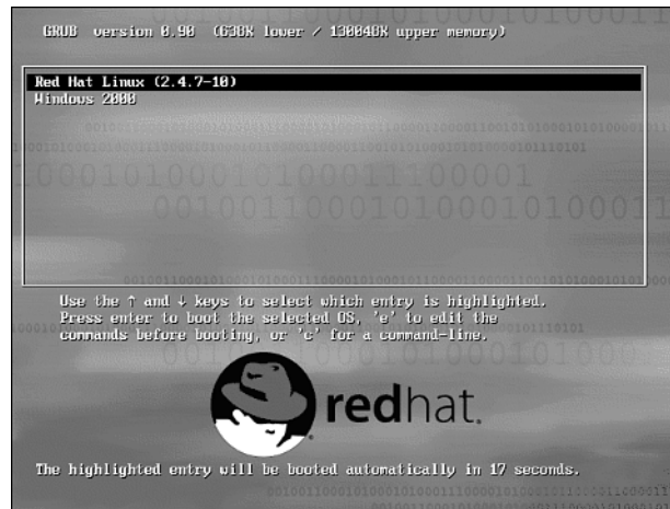
FIGURE 11.1 GRUB boot screen with two operating systems.
