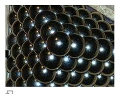
Model of closely packed atoms within a crystalline solid.
