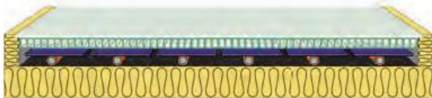
collector with transparent heat insulation
