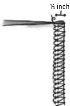
Figure 6-11: \frac{1}{4} -inch seam sewn with a four-thread overlock stitch on the serger.
