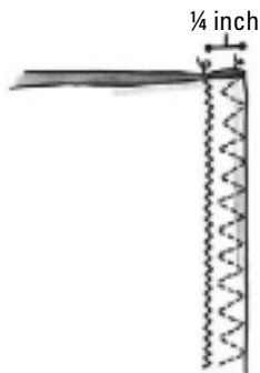
Figure 6-10: Two-step \frac{1}{4} -inch seam.
