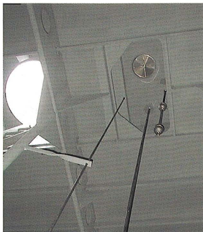
Cargo tank zone 0 with level sensors
