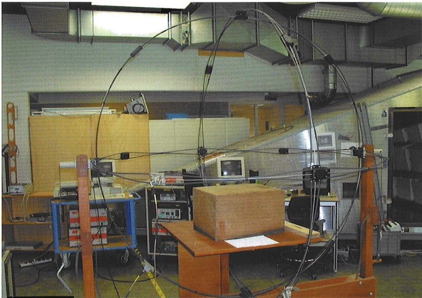
Radiated and conducted interference (EMC Susceptibility) is tested in a special created environment.
