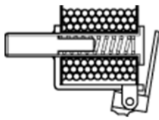
Fig. F-3-5-2(b) Current within rating – magnetic field insufficient to attract tripping armature or to move core
