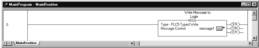
Figure 7.8 Example of a Write MSG from a Logix to a Logix Controller
