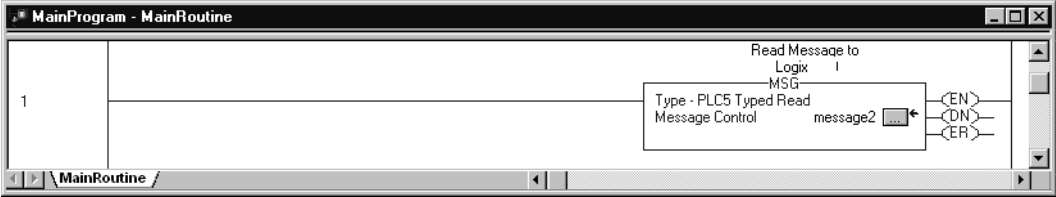
Figure 7.9 Example of a Read MSG from a Logix to a Logix Controller
