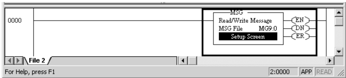
Figure 3.7 Write MSG from an MicroLogix 1100/1200/1500 controller to a PLC-5 Processor or Logix Controller
