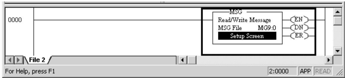
Figure 3.8 Read MSG from a MicroLogix 1100/1200/1500 controller to a PLC-5 Processor or Logix Controller.
