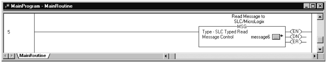
Figure 7.13 Read MSG Instruction from a Logix to an SLC or MicroLogix Controller
