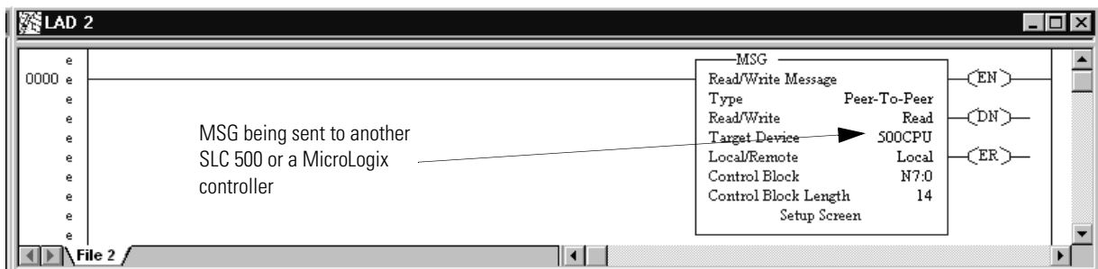
Figure 4.9 Read MSG from an SLC 5/03, 5/04, or 5/05 Processor to Another SLC 500 or MicroLogix Controller
