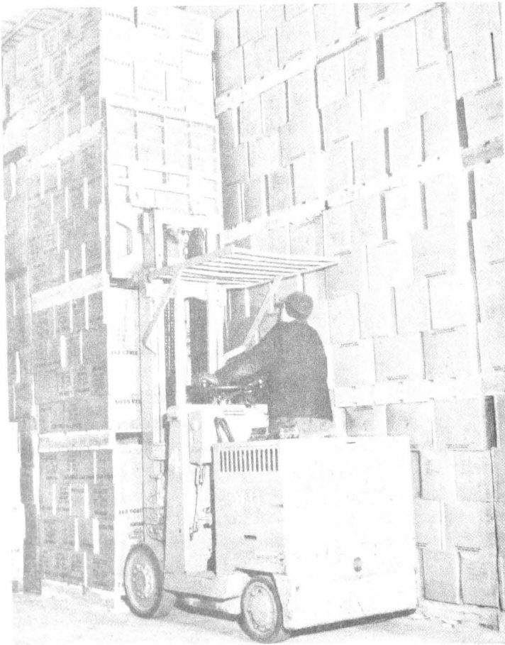
Figure 4.--A fork lift truck handling frozen products in a refrigerated warehouse. (Photo courtesy of Quincy Market Cold Storage and Warehouse Co.)
