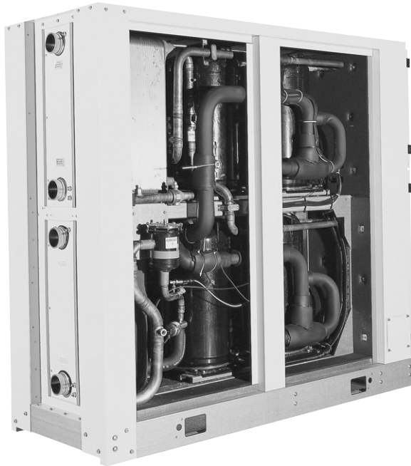
Figure 13.8 Water-cooled water chiller, nominal 250 kW capacity with two R407C refrigerant circuits, brazed plate heat exchangers (1 evaporator, 2 condensers), and multiple scroll compressors (Airedale)
