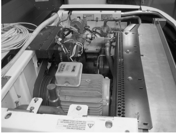
Figure 17.5 Self powered diesel truck unit with electric standby option (Thermo King)
