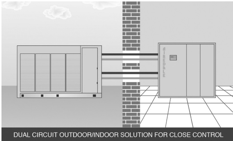
Figure 13.9 Dual circuit split system package, outdoor air-cooled condensing unit with scroll compressors matched with indoor evaporator unit, typically 50–80 kW capacity (Airedale)
