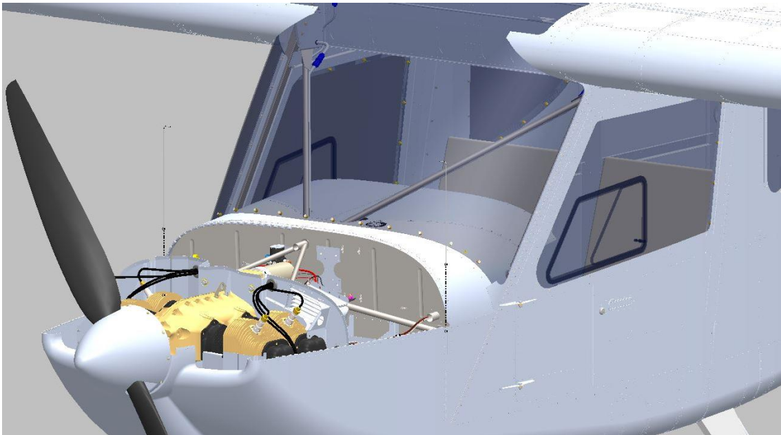
Figure 5.7.9.6 Lower cowl hinge pin removal.
