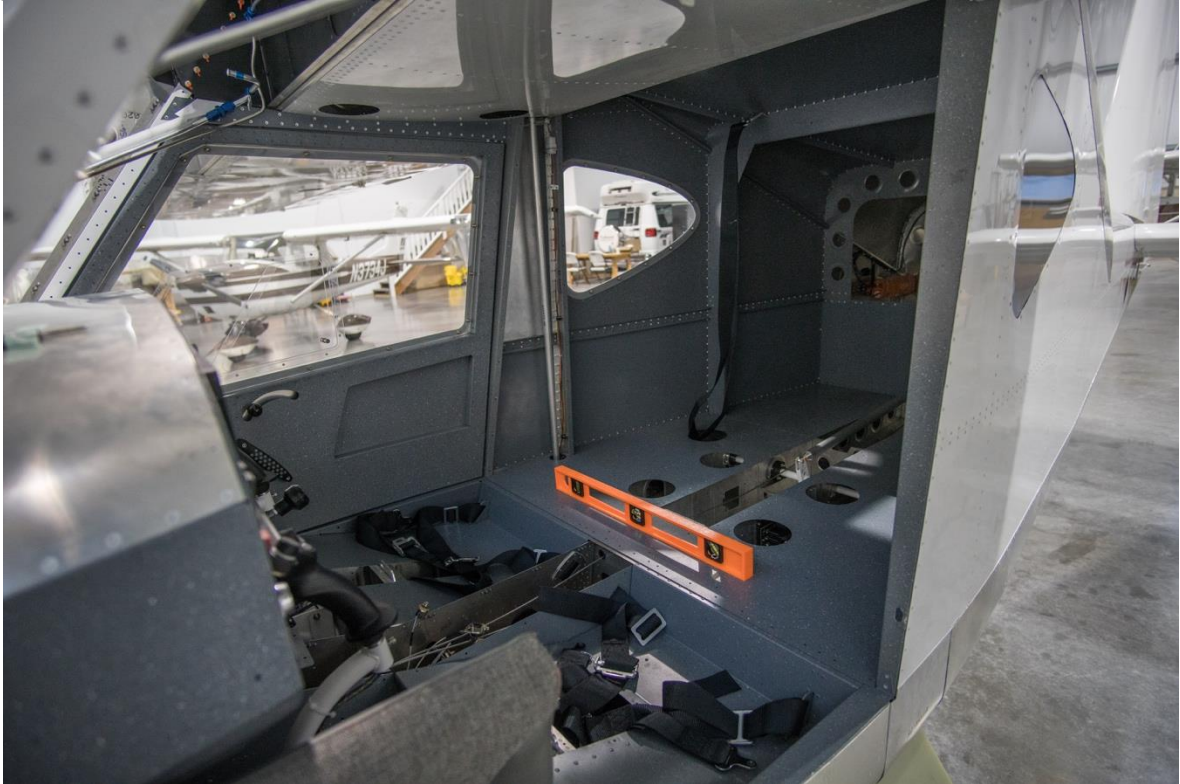
Figure 5.7.24.2 Lateral leveling of the aircraft.
