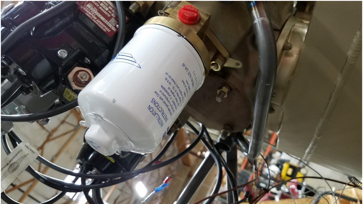
Figure 5.7.10.1 Oil filter secured by safety wire.
