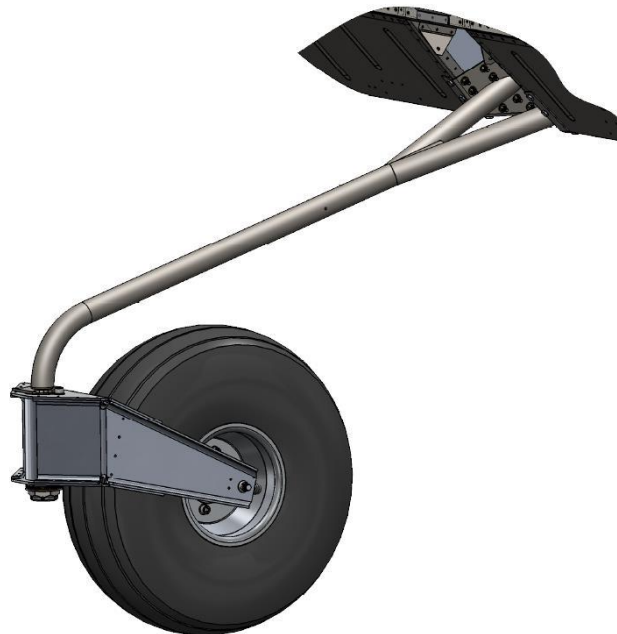
Figure 5.7.7.1 The main landing gears with fuselage skin hidden for clarity.
