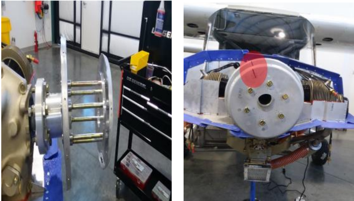
Figure 5.7.16.7 Front spinner bulkhead alignment.
