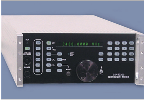
CS-5020C-series microwave tuners and receivers are high-performance instruments covering the centre tune frequency range from 0.1-18GHz. (Photo: Collins Aerospace)
