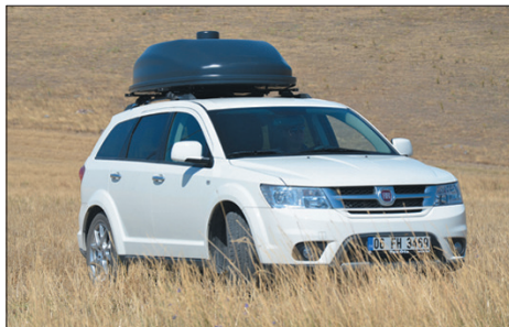
The Mobile Direction Finding system components are integrated onto a 4x4 vehicle with disassembly possibility. (Photo: Aselsan)
