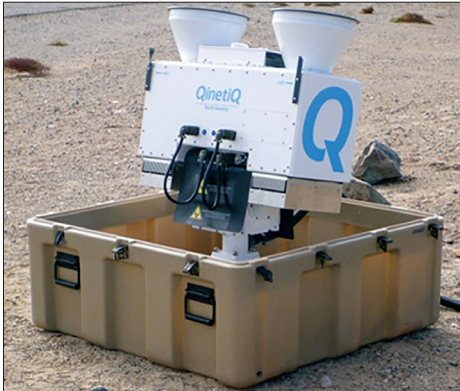
QinetiQ North America's WiPPR has been designed to provide near-real-time wind measurements for a variety of applications. (Photo: QinetiQ North America)
