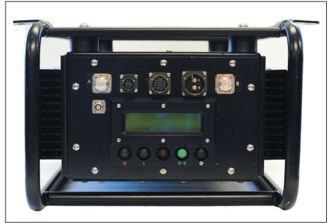
The 3XXX ECM suite is a combination system based on the fully programmable 3140 and 3230 ECM units. (Photo: Allen-Vanguard Canada)
