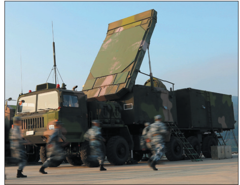
The CPMIEC HT-233 fire control radar is designed to detect and track flying targets and is associated with HQ-9 and HQ-10 surface-to-air missile batteries. (Photo: CPMIEC)
