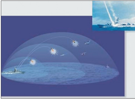
Rafael's integrated ship-defence decoy system features real-time decoy deployment, fixed and/or rotating launchers and a computerised decoy controller. (Image: Rafael Advanced Defense Systems)
