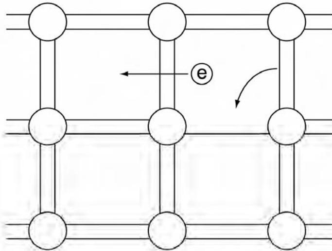
Figure 2.1. Schematic representation of covalent bonds in a silicon crystal lattice.
