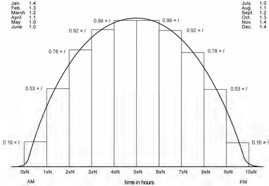
Figure H.2. Profile of light intensity throughout a typical sunny day, as a function of the peak daily intensity  $I$ . The histograms of width  $N$  represent an approximation to the daily light intensity profile, with  $N$  being determined by the time of the year.
