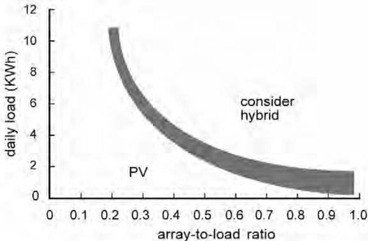
Figure 7.2. The *hybrid indicator* (Sandia National Laboratories, 1991).
