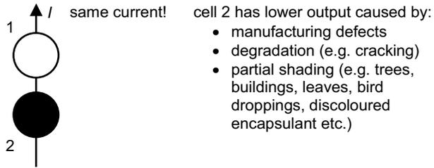
Figure 5.5. Mismatched cells connected in series.
