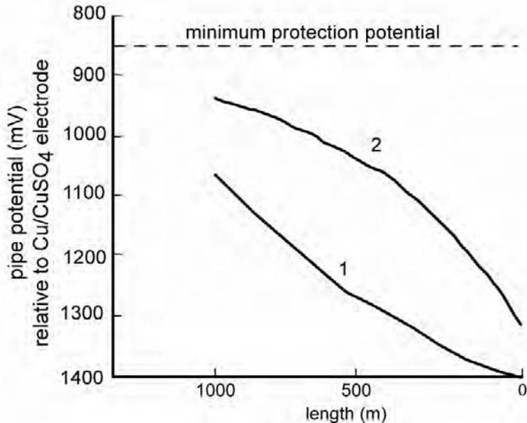
Figure 8.3. Typical pipe potential distribution for a sunny day (curve 1), and at night following a cloudy day (curve 2) (Tanasescu *et al*, 1988, Used with kind permission from Springer Science and Business Media).
