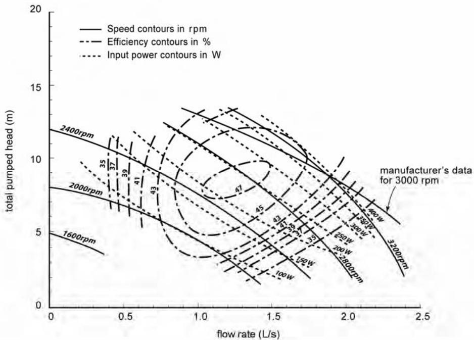
Figure H.4: Centrifugal pump with performance characteristics and pumping rates suited to the specification (Used with permission of Halcrow & Partners, 1981).
