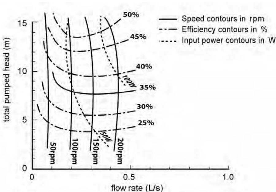
Figure 11.8. Performance curves of a typical positive displacement pump. (Speeds shown are pump speeds. For motor, multiply by 8.5. Efficiencies include belt transmission between motor and pump.) (Used with permission of Halcrow & Partners, 1981).
