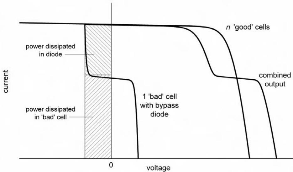
Figure 5.13. Effect on total output of a 'bad' cell with a bypass diode. When the combination is short-circuited, the total power dissipated in the bad cell and bypass diode is approximately equal to the output capability of one good cell.
