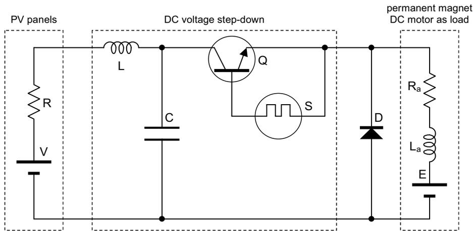
Figure 11.16. Simple DC-to-DC converter (Kheder & Russell, 1988, Used with kind permission from Springer Science and Business Media),  $R$  = resistor,  $V$  = voltage source,  $L$  = inductor,  $C$  = capacitor,  $Q$  = transistor,  $S$  = control signal,  $D$  = diode,  $R_a$  = armature resistance,  $L_a$  = armature inductance,  $E$  = motor back emf.
