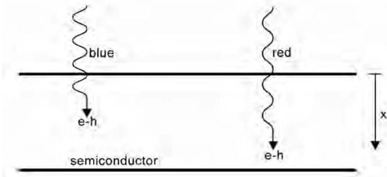
Figure 2.7. The light energy dependency of electron-hole generation.
