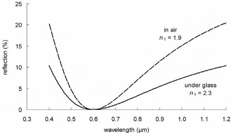
Figure 4.3. Surface reflection from a silicon cell ( $n_2 = 3.8$ ) in air ( $n_0 = 1$ ) and under glass ( $n_0 = 1.5$ ) with an antireflection coating with refractive index and thickness chosen so as to minimise reflection for  $0.6 \mu\text{m}$  wavelength light.
