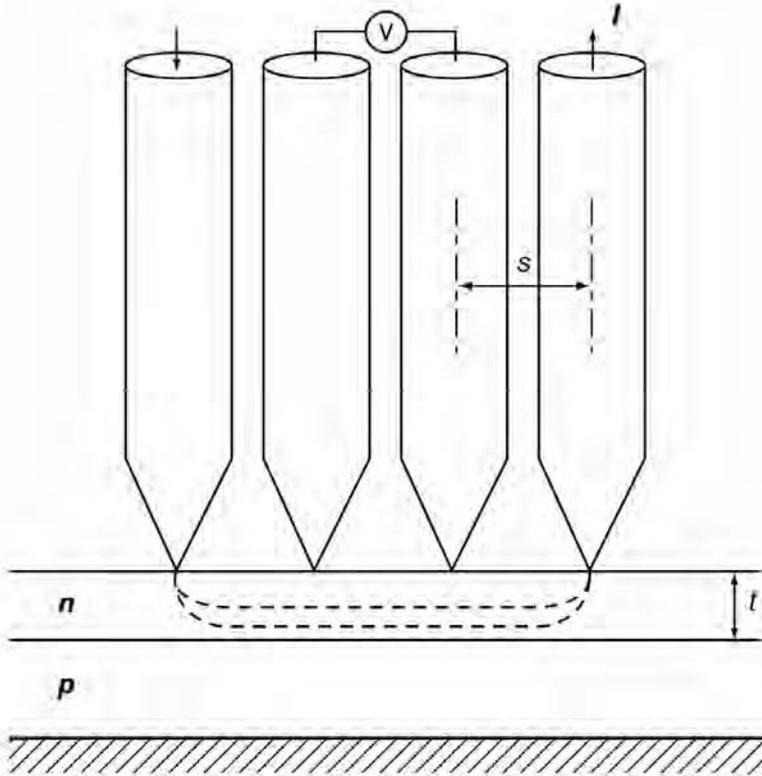
Figure 4.12. Use of a four point probe to measure the sheet resistivity of a solar cell.
