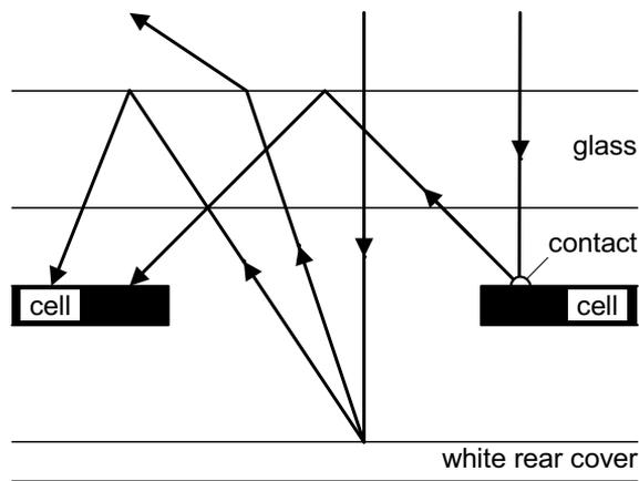
Figure 5.21. The *zero-depth concentrator effect* in modules with sparsely packed cells and a white rear surface.
