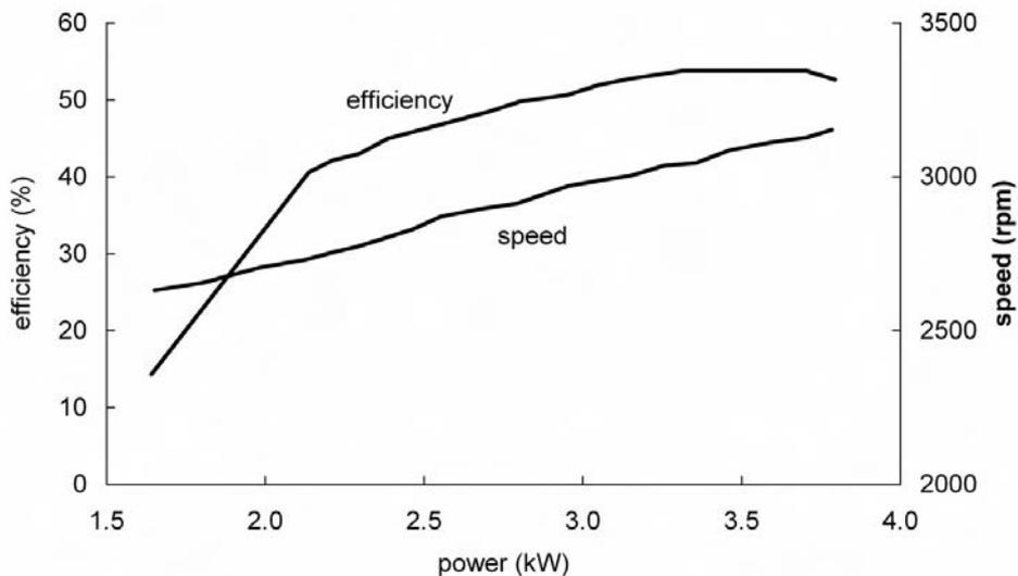
Figure 11.6. Typical efficiency characteristics of a centrifugal pump at variable speed (60 m head, 10 m<sup>3</sup>/h flow rate, 3 kW power). (Used with permission of Thomson, Landau, M., Sachau, J. & Raatz, A. (1992), 'Photovoltaic pumping system for intermittent operation', Proc. 11th EC Photovoltaic Solar Energy Conference, Montreux, Switzerland, pp. 1391–1394, Fig.1, Published by Taylor & Francis 1993)
