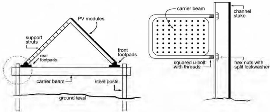
Figure 6.7. Simple ground mounting for PV arrays using materials readily available from a hardware store (reprinted with permission of Sandia National Laboratories, 1991).
