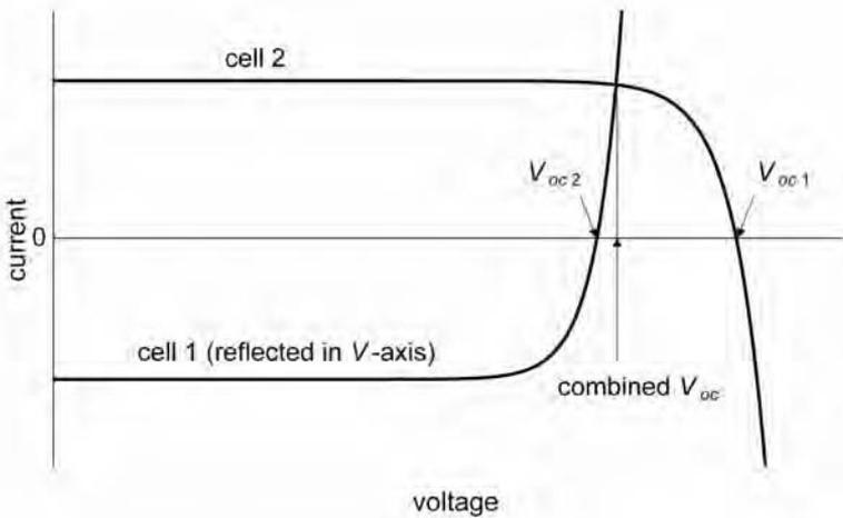
Figure 5.4. An easy method of calculating the combined  $V_{oc}$  of mismatched cells in parallel. The curve for one of the cells is reflected in the voltage axis so that the intersection point (where  $V_1 + V_2 = 0$ ) is the  $V_{oc}$  of the parallel configuration.
