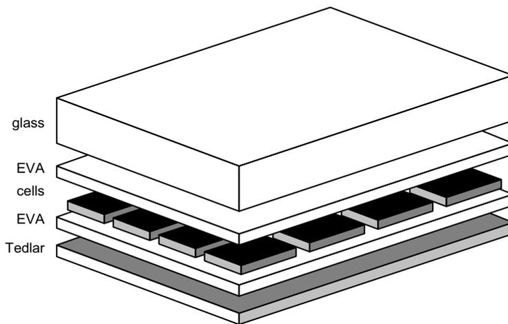
Figure 5.17. A typical laminated module structure.
