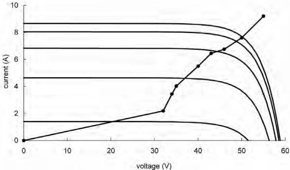
Figure H.5. I-V curves corresponding to the daily insolation profile, as given by Fig. H.2 for the month of December, with the motor-pump load line from Table H.4 superimposed.
