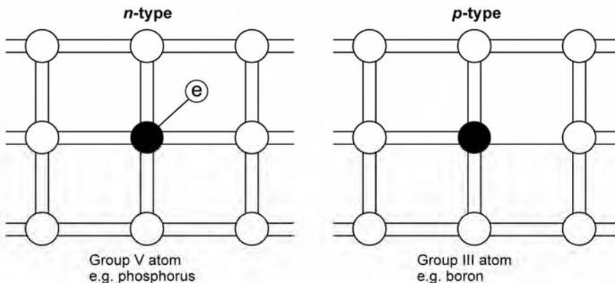
Figure 2.3. Schematic of a silicon crystal lattice doped with impurities to produce *n*-type and *p*-type semiconductor material.
