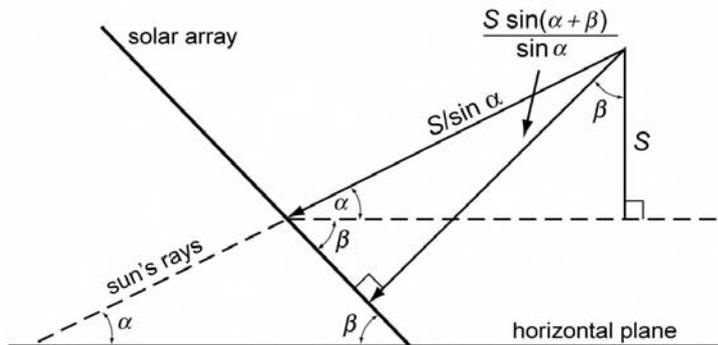
Figure 1.15. Light incident on a surface tilted to the horizontal (after Mack, 1979).
