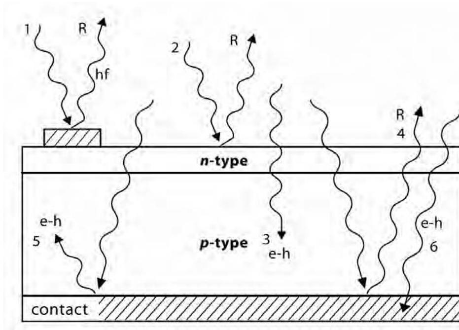
Figure 3.1. Behaviour of light shining on a solar cell. (1) Reflection and absorption at top contact. (2) Reflection at cell surface. (3) Desired absorption. (4) Reflection from rear out of cell—weakly absorbed light only. (5) Absorption after reflection. (6) Absorption in rear contact.
