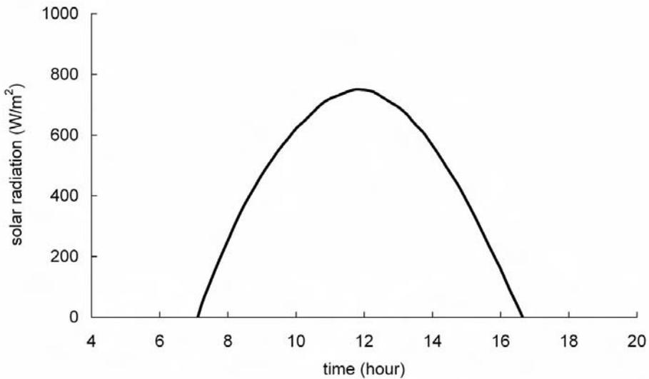
Figure 11.18. Solar radiation received on an inclined plane throughout a clear sunny day.
