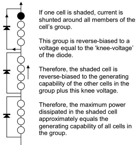
Figure 5.14. Bypass diodes used across groups of cells in a module.
