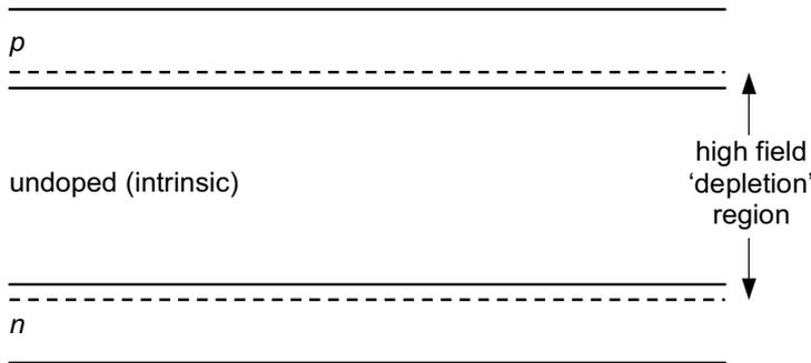
Figure 2.5. Schematic of an a-Si:H solar cell.
