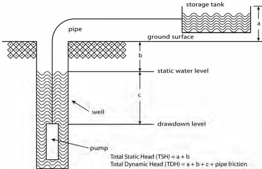
Figure 11.1. Common water pumping terms (after Sandia National Laboratories, 1991, used with permission).
