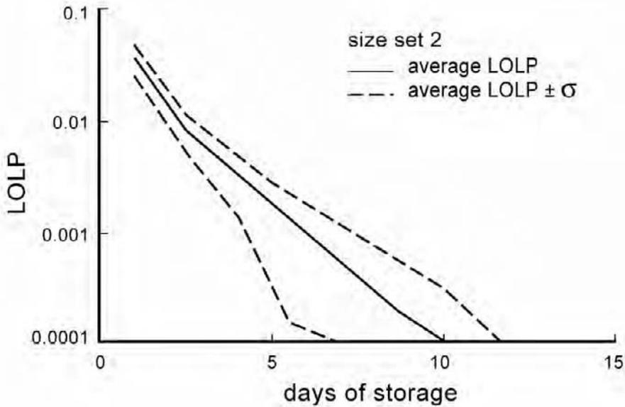
Figure G.1. Number of days of battery storage as a function of *loss-of-load probability* for design 2 (©1987 IEEE, Chapman).
