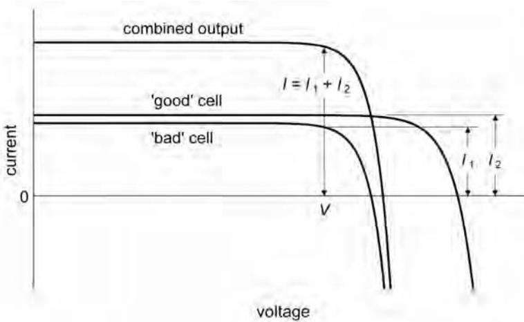
Figure 5.3. Parallel-connected mismatched cells and the effect on current. The combined curve is determined by summing the currents  $I_1$  and  $I_2$  for each voltage  $V$ .
