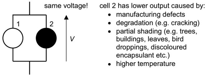
Figure 5.2. Mismatched cells connected in parallel.
