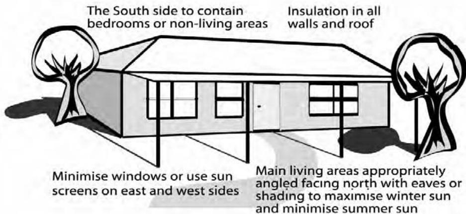
Figure 9.1. A home based on energy efficient passive solar design principles for the southern hemisphere. The directions north and south are reversed for the northern hemisphere.
