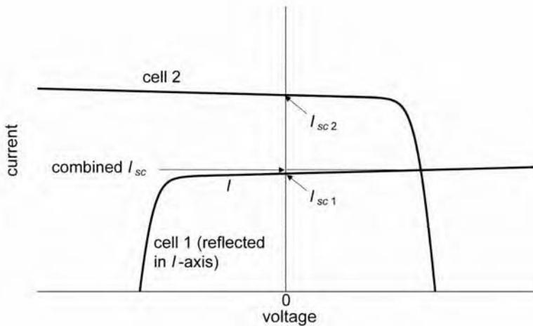
Figure 5.7. An easy method of calculating the combined  $I_{sc}$  of series-connected mismatched cells. The current at the point of intersection represents the short circuit current of the series combination (i.e.  $V_1 + V_2 = 0$ ).
