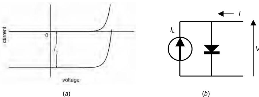
Figure 3.4. The effect of light on the current-voltage characteristics of a  $p$ - $n$  junction.
