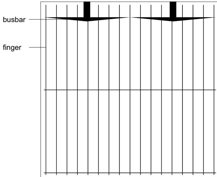
Figure 4.10. Top contact design of a solar cell.
