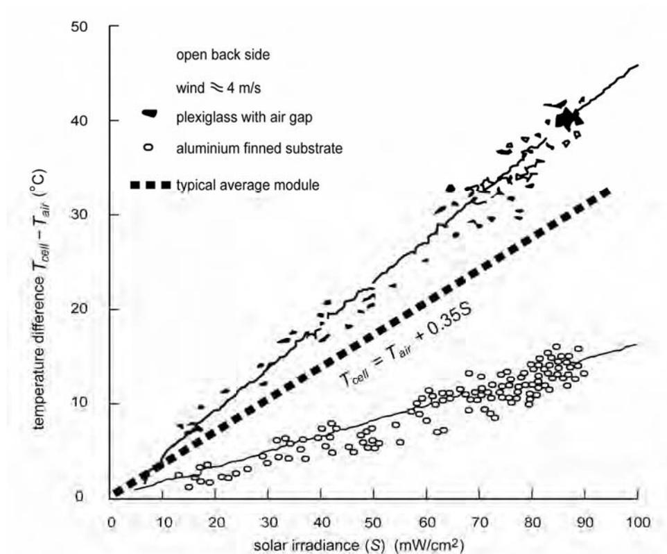
Figure 5.19. Temperature increases, above ambient levels, with increasing solar irradiance for different module types (Ross & Smokler, 1986).
