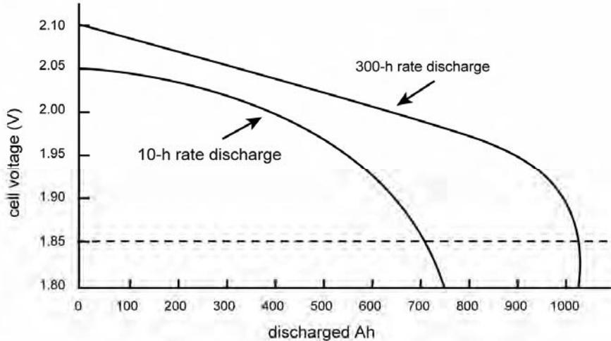
Figure 6.4. Constant-current discharge curves for a 550 Ah lead-acid battery at different discharge rates, with a limiting voltage of 1.85 V per cell (Mack, 1979; reprinted with permission of the Telecommunication Society of Australia).
