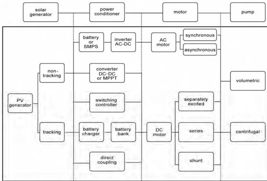
Figure 11.2. Photovoltaic water pumping system components and configurations (Used with permission of Regional Energy Resources Information Centre, Koner, 1993).
