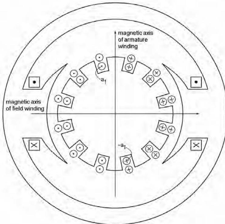
Figure 11.13. Cross-section of a two-pole DC machine (Used with permission of McGraw-Hill Companies, adapted from Fitzgerald, A.E., Kingsley C. Jnr. & Kusko, A. (1971), *Electric Machinery*, McGraw Hill, Tokyo, Japan).
