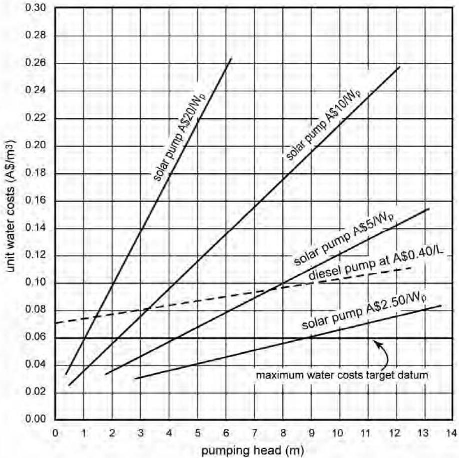
Figure 8.6. Typical unit water costs as a function of pumping head for 40 m<sup>3</sup>/day average pumping output (Used with permission of Halcrow & Partners, 1981).
