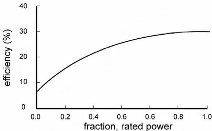
Figure 9.4. Diesel generator efficiency as a function of load.
