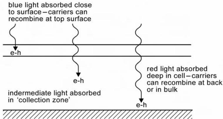
Figure 4.8. Possible sites for recombination of e-h pairs within a PV cell.
