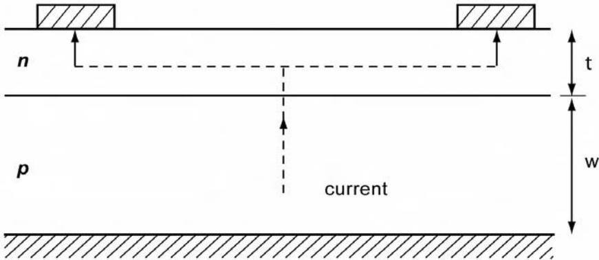
Figure 4.11. Current flow from point of generation to external contact in a solar cell.
