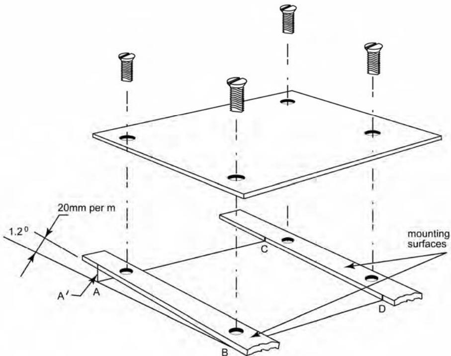
Figure 5.23. Possible module twisting on a distorted mounting frame (JPL, 1981).
