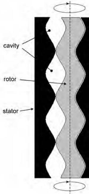
Figure 11.7. Helical rotor type of displacement pump (after Revard, 1995).
