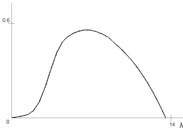
Fig. 5.8. Power coefficient for a 3-blade rotor
