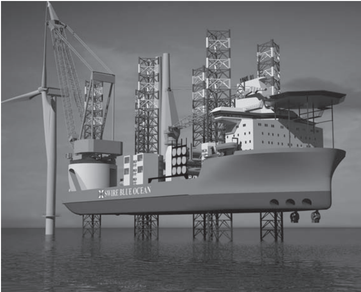
Figure 8.6 Example of a mobile jack-up installation [Source: Swire Blue Ocean]
