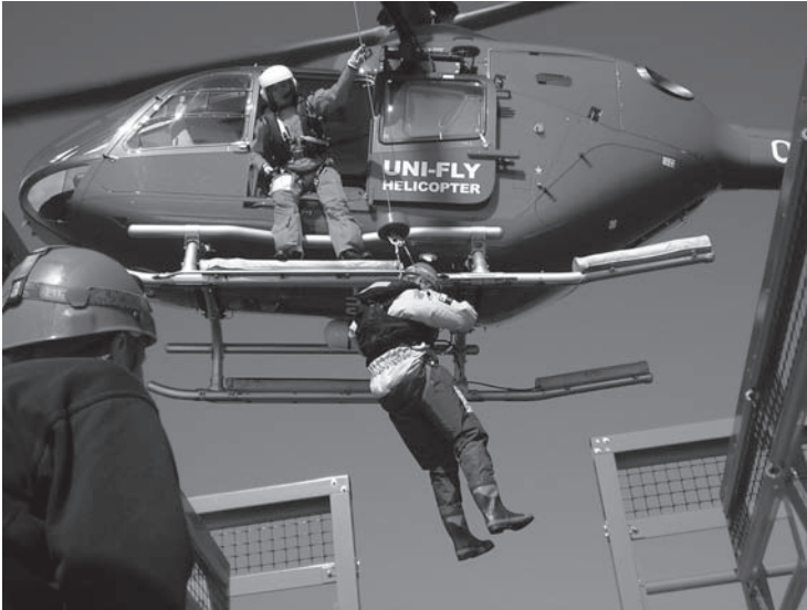
Figure 8.4 Example of offshore access to Vestas V80 WT's at Horns Rev by Eurocopter EC135 [Source: Unify]
