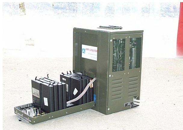
Figure 5.32. Walkie-talkie battery recharging unit
