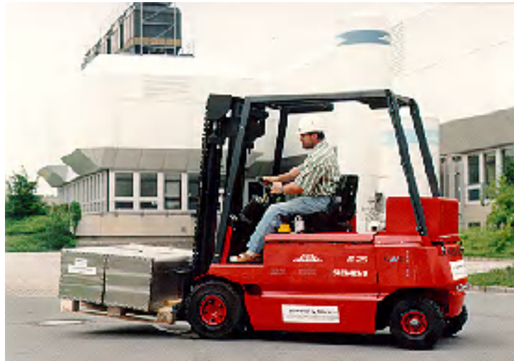
Figure 5.37. Siemens forklift truck powered by a PEMFC
