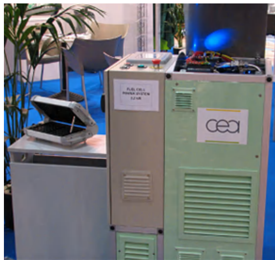
Figure 5.42. Motor generator set fuel cell of 3.2 kW developed by the CEA
