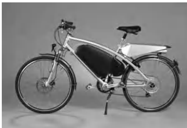
Figure 4.11. Masterflex hydrogen fuel cell motor cycle with a 120 km range (Germany, 2005)
