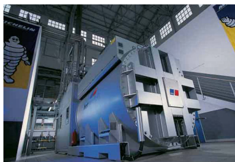
Figure 5.45. MCFC developed by MTU: 250 kW e + 180 kW th
