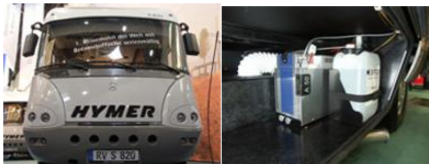
Figure 5.36. DMFC as APU on Hymer motor home (2005)
