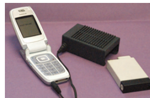
d) Disposable H 2 cartridge with sodium borohydride for miniatures fuel cells developed at the CEA
