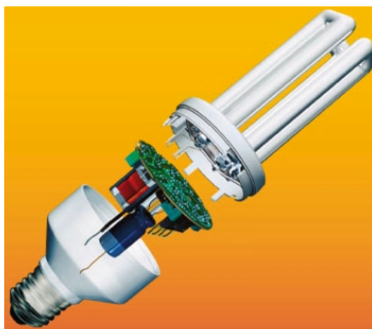
Figure 7.9. Compact fluorescent lamp (CFL) with its integrated electronic ballast (with the permission of Osram GmbH)
