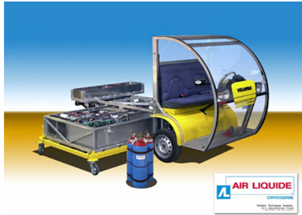
Figure 5.39. Velapac prototype of a utility vehicle for use in a post office
