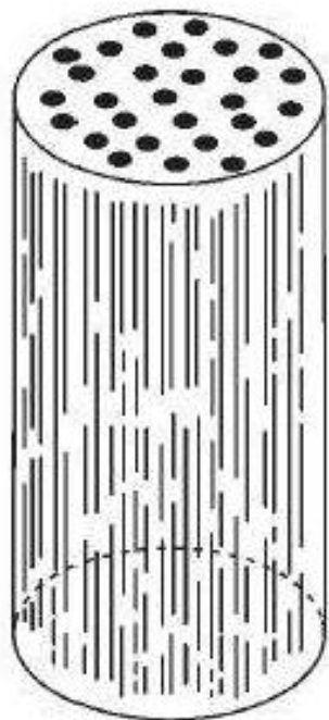
Figure 24.2 Composite rod with long parallel fibres.
