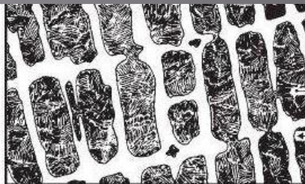
(i) White cast iron (low silicon) – primary cementite network in a matrix of pearlite.
