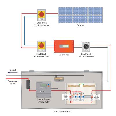
Arrange the following items into the correct order to create a commissioning procedure, complying with AS/NZS 5033:2021 and AS/NZS 3000:2018, for the grid-connected PV installation pictured above.
