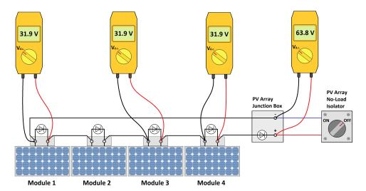
The diagram above shows a PV array, consisting of four 180 W modules, undergoing voltage testing. What do the test results indicate?
