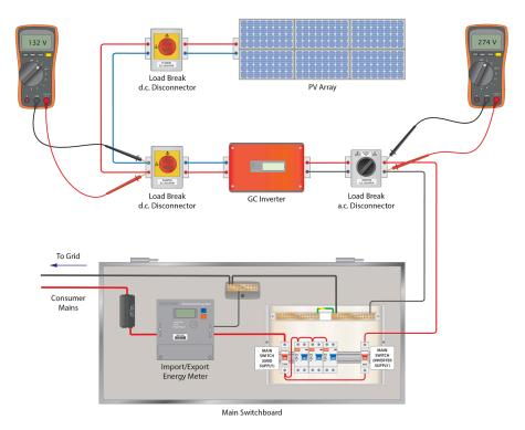
The power output of the PV array pictured above has dropped to zero. When the current was measured in the positive conductor running between the d.c. isolator and the GC inverter, a reading of zero amperes was taken.
