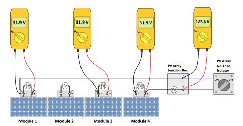
The diagram above shows a PV array, consisting of four 145 W modules, undergoing voltage testing. What do the test results indicate?
