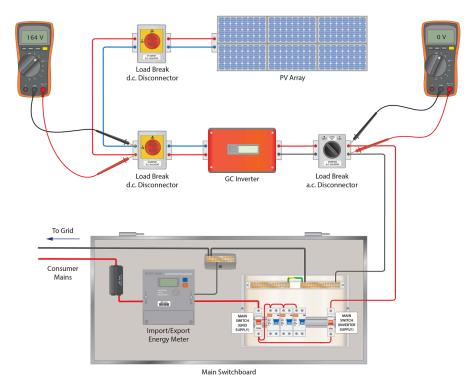
The power output of the PV array pictured above has dropped to zero. Given the voltage measurements indicated, what is the most likely root cause of the problem?
