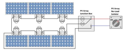
The PV array pictured above consists of six modules, each having a maximum voltage (VMOD MAX) of 45 V d.c.. In order to verify the insulation resistance of the array interconnect wiring:
