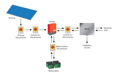
In relation to the installation pictured above, which disconnectors (isolators) need to be locked out and tagged, as a minimum, so that repair work can be safely carried out on the inverter?
