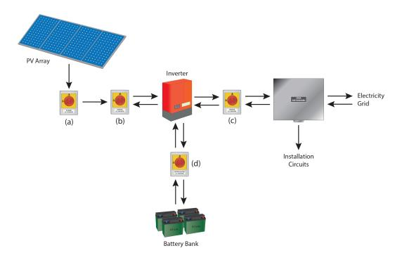
In relation to the installation pictured above, which isolators need to be locked out and tagged, as a minimum, so that repair work can be safely carried out on the inverter?
