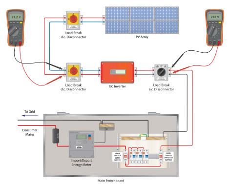
Examine the diagram above, showing a 1.2 kW PV system, having a nominal voltage of 72 V d.c.
