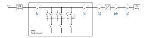
Which of the following labels is suitable for identifying switch (b) in the grid-connected PV installation pictured above?
