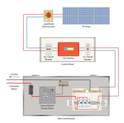
Arrange the safe isolation procedure into the correct sequence, to carry out routine maintenance on the PV array pictured above.
