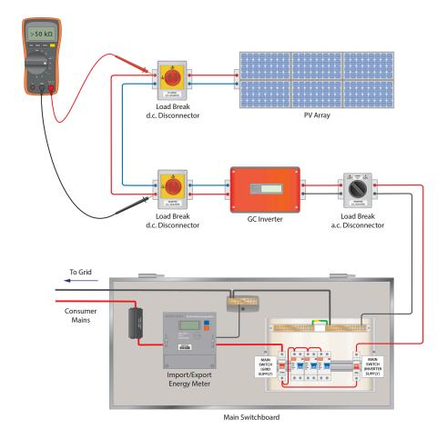
Examine the diagram above, showing the active conductor of the d.c. cabling between the array and the inverter under test during system commissioning.
