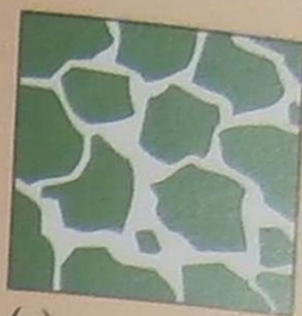
(c) medium porosity – angular grains, uniform size (good sorting)
