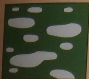
(e) vesicular porosity – may not be interconnected, e.g. basalt
