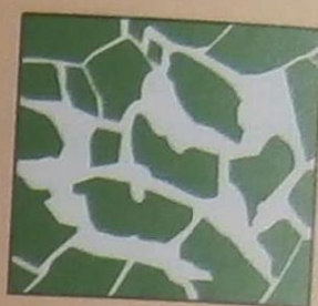
(f) solution porosity – mild solution along crystal boundaries e.g. limestone
