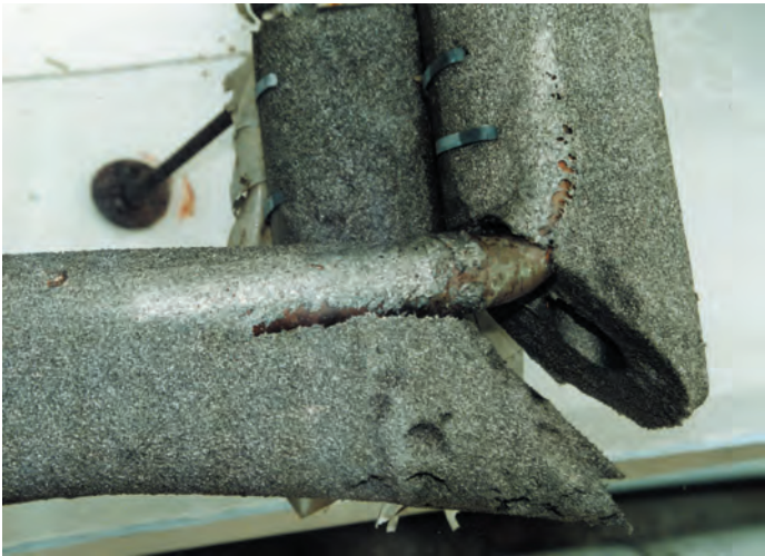
Figure 4.53 Damaged thermal insulation
