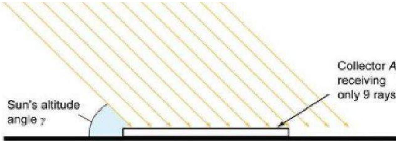
**Figure 2.21** If the same collector is laid horizontally on the Earth's surface at the same time as in the image above, the collector only captures 9 rays
