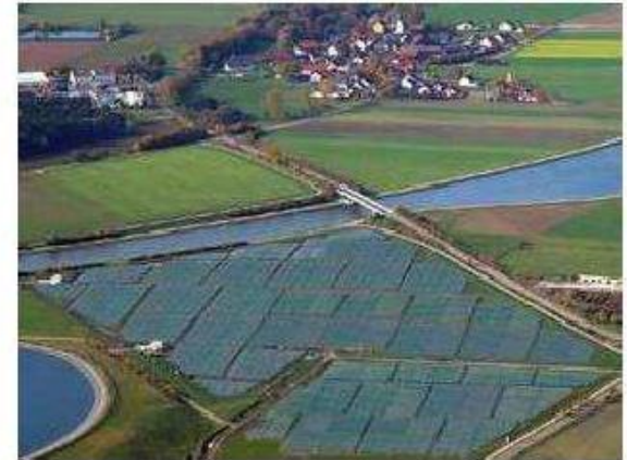
Figure 6.7. A solar photovoltaic farm: the 6.3 MW (peak) Solarpark in Mühlhausen, Bavaria. Its average power per unit land area is expected to be about 5 \text{ W/m}^2 . Photo by SunPower.
