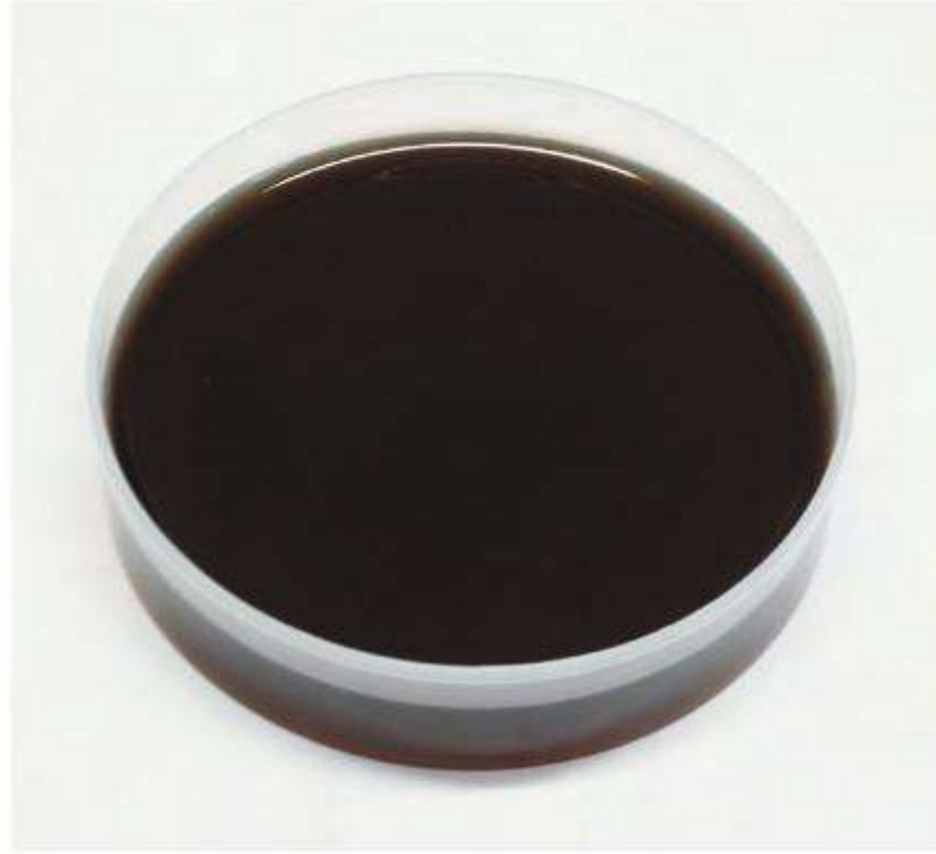
Figure 4.55 Damaged propylene glycol
