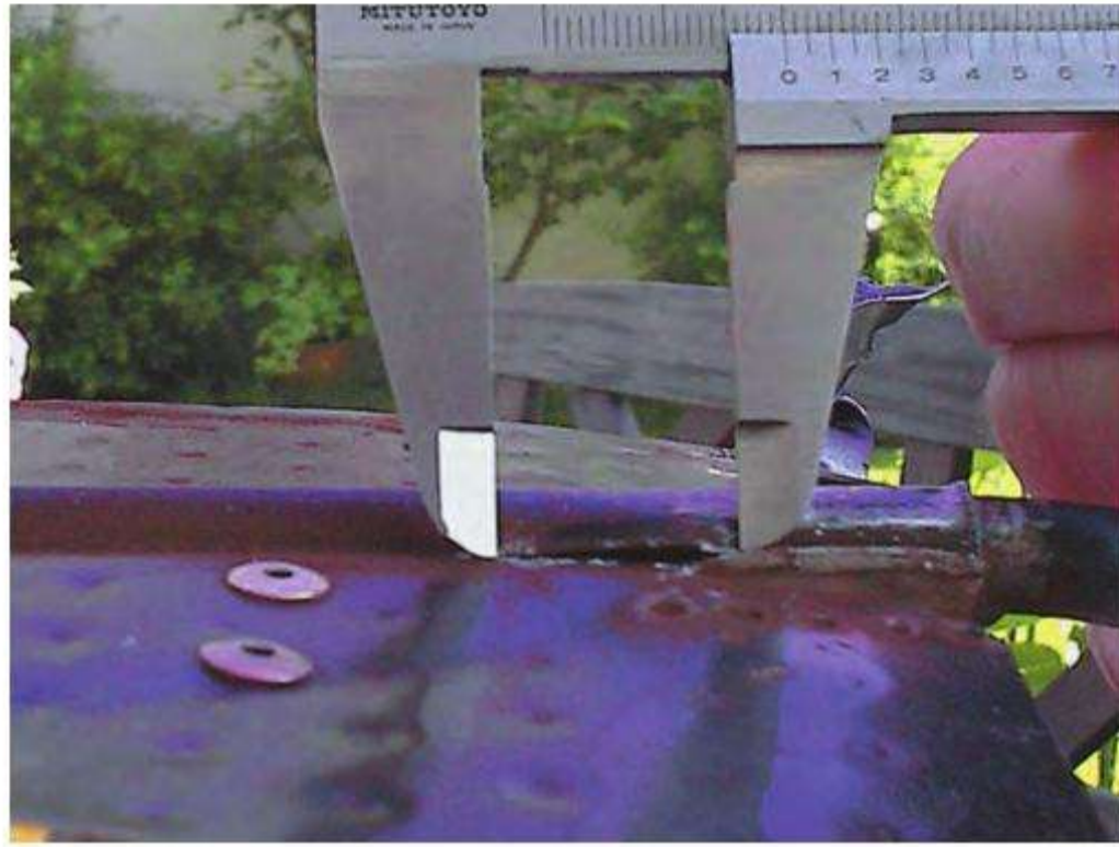
Figure 4.52 Break by ice formation
