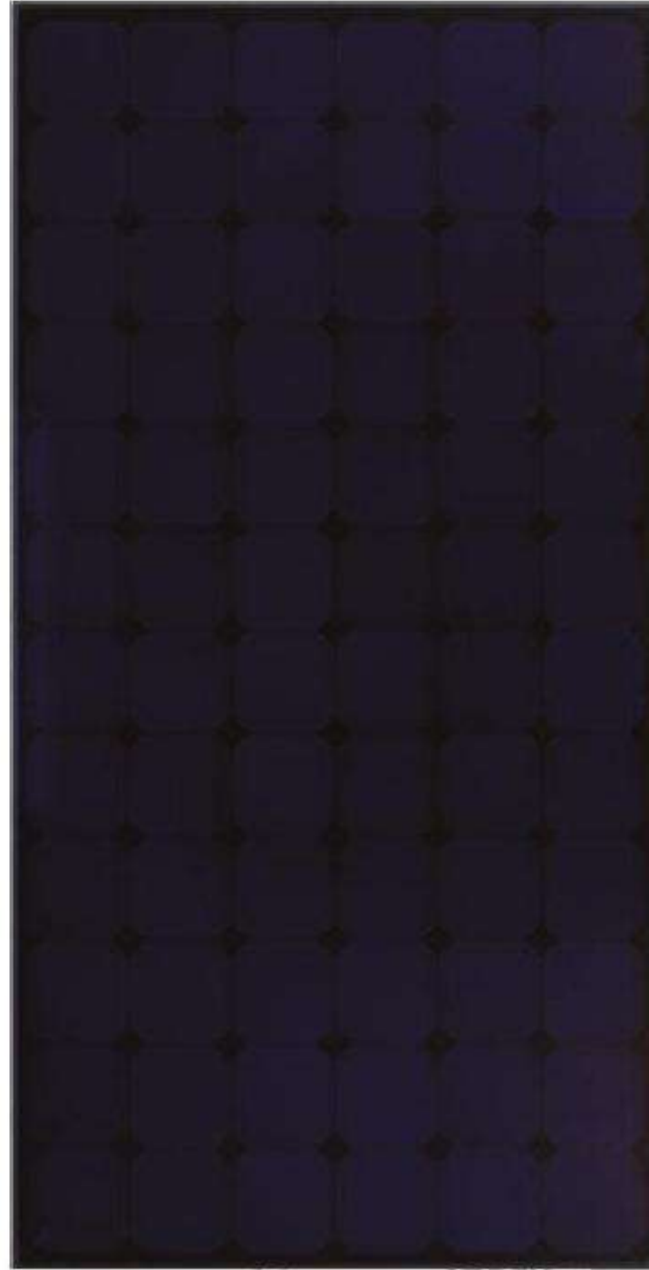
Figure 8.1 There are several module types on the market that are all (or mostly) black. It should be kept in mind that crystalline modules with a black backing sheet will have a higher effective cell temperature and therefore lower power output than the same module with a white backing sheet
