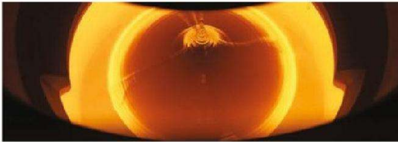
Figure 3.2 A single-crystal silicon ingot is drawn from the molten silicon
