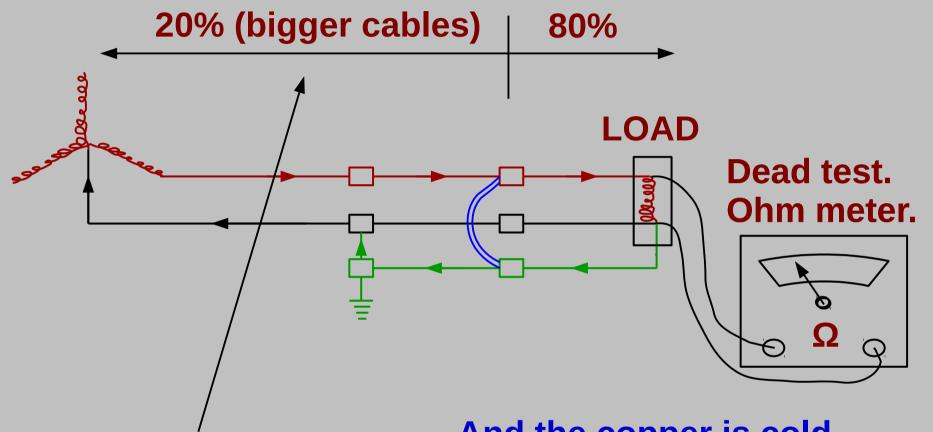
However this method does not test 20% of the circuit And the copper is cold when tested and could have a higher resistance when operating at 75°
