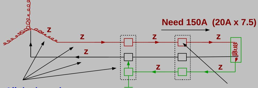
All the impedances added together makes the Fault-Loop Impedance
