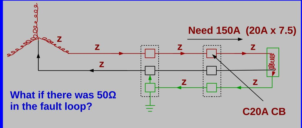
$I_{a} = \frac{V}{Z} = \frac{230 V}{50 \Omega} = 4.6 A$  $4.6 A = 0 \times \text{Overload}$
