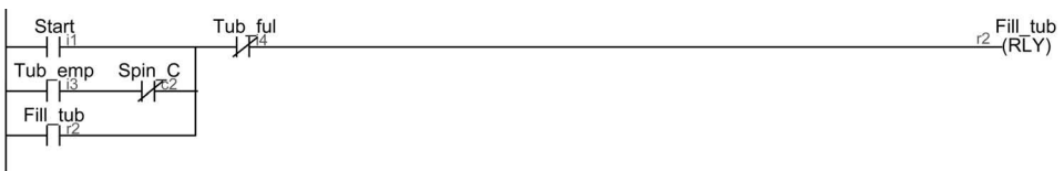
Figure 9-72 Fill tub state transition logic
