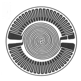
Figure 9-14 - Diaphragm Strain Gage (Omega Instruments)
