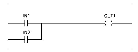
Figure 5-3 - Ladder Diagram for OR Function
